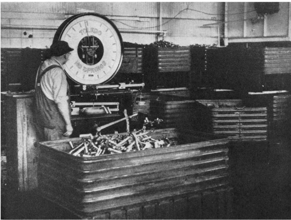
Counting by weight. Bin in foreground is on scale platform; number of items in scale pan, multiplied by the scale reading, gives number of items in bin
