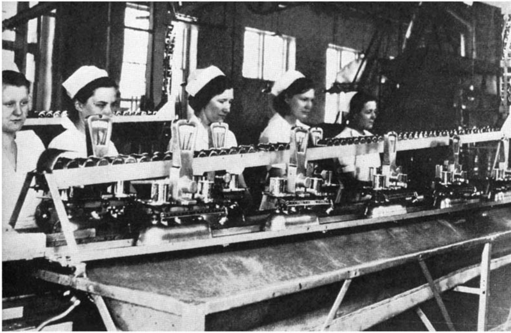
A battery of scales at this filling table in a mushroom packing plant makes it possible for the operators rapidly to fill each of the cans with exactly the same quantity of the delicacies
