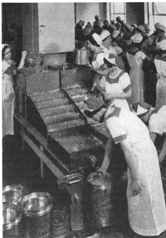
Millions of egg whites are yearly distributed to large users. Here they are being canned and weighed in one operation through use of floor-type scales fitted with top-reading dials
