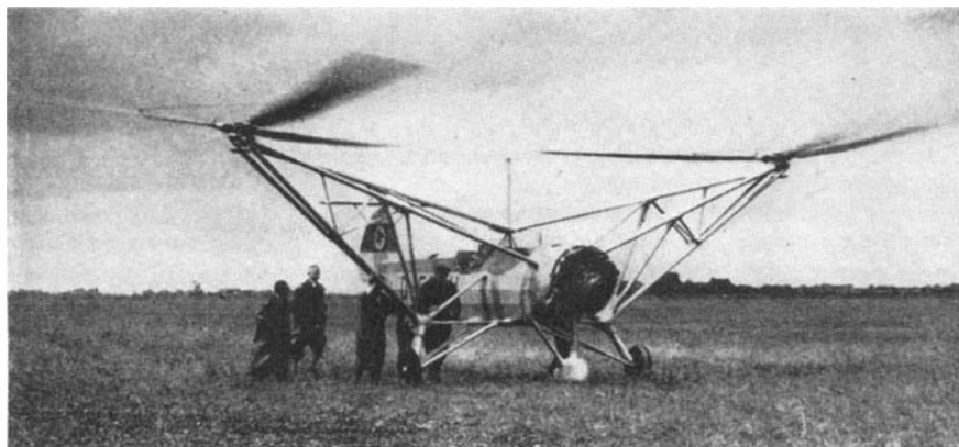
Front view of the Focke helicopter with lifting screws in rotation
