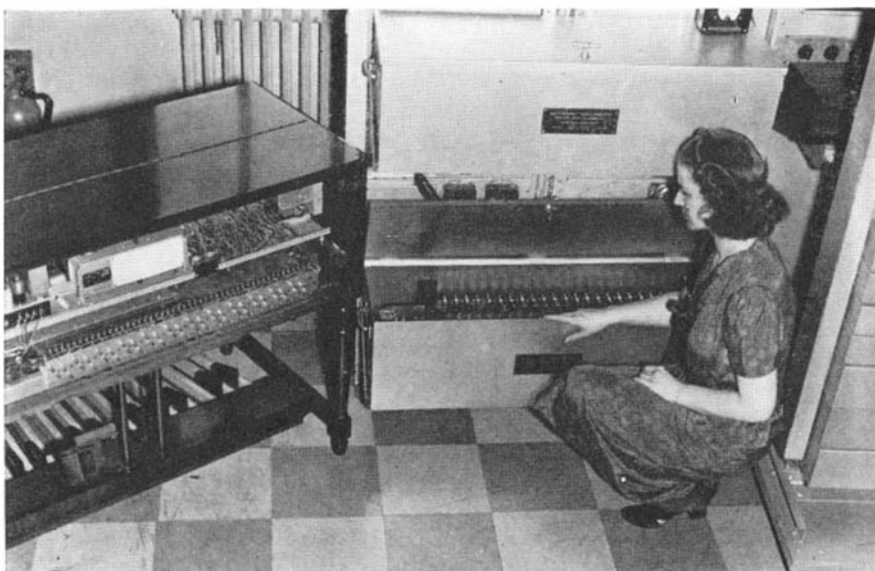
Tone generator of Hammond organ, left , and of telegraph equipment, right
