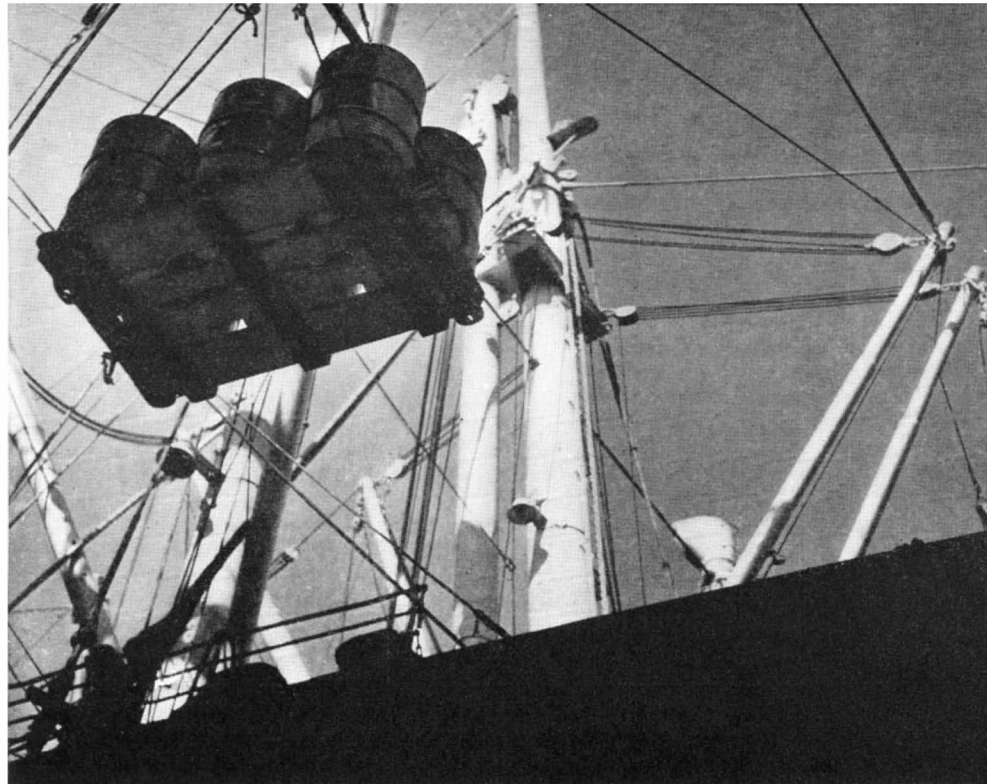
For hoisting aboard liquid-filled barrels, perhaps those shown in the opposite photograph, spreader bridles and skids, upon which the barrels rest, are used as in the illustration above
