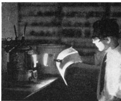
The high-temperature electric arc furnace when in actual operation
