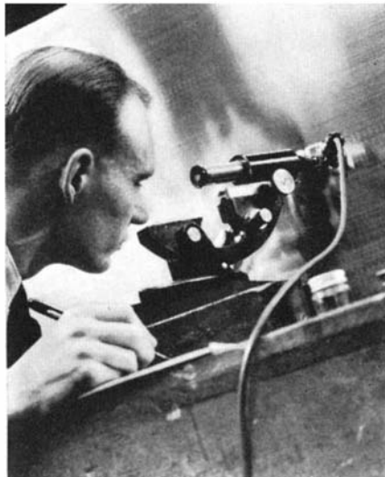
Checking surface of giant bearing
