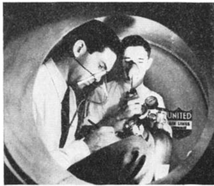
Above: The stratosphere laboratory test chamber for aeronautical research. Left: Oxygen-inhaling apparatus being put through its paces under simulated altitude conditions
