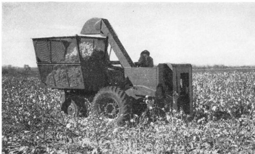
Another view, from the left rear, of a slightly different form of cotton picker made by International Harvester Company
