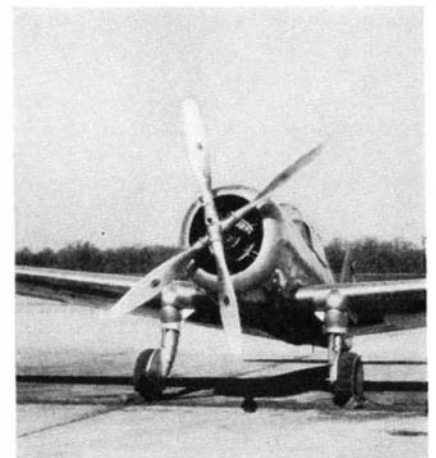
One engine drives the two propellers rotating in opposite directions
