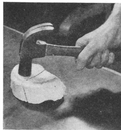
Repeated hammer blows are necessary to break boric oxide crystals
