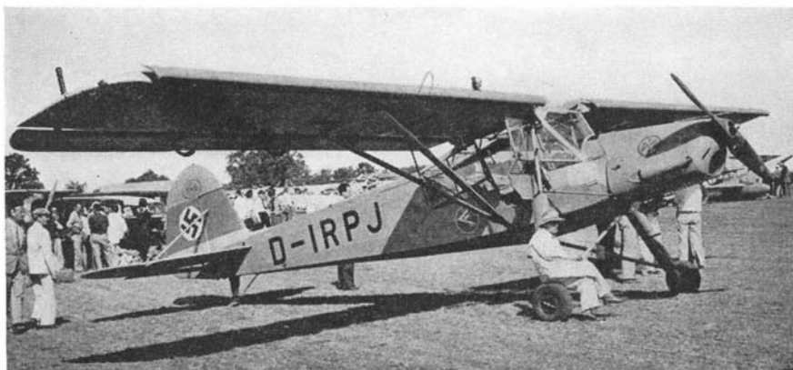
The Fieseler-Storch, a German monoplane with slots and flaps, which recently created a sensation by its ability to fly and land slowly, under perfect control
