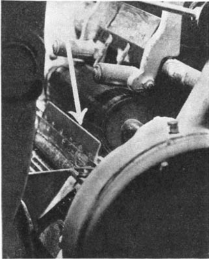
The dough scraper, hard-faced, in long service without reconditioning
