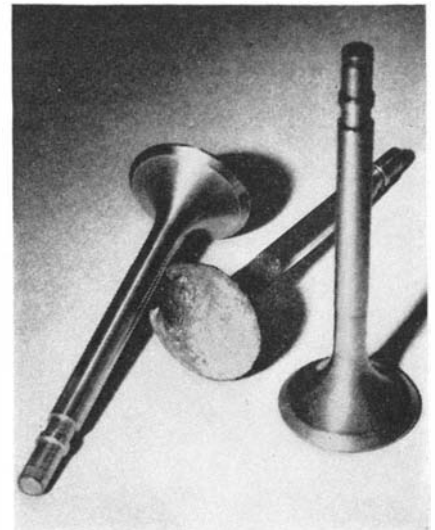
Hard-faced valve at right after 650 hours; center, steel after 150 hours
