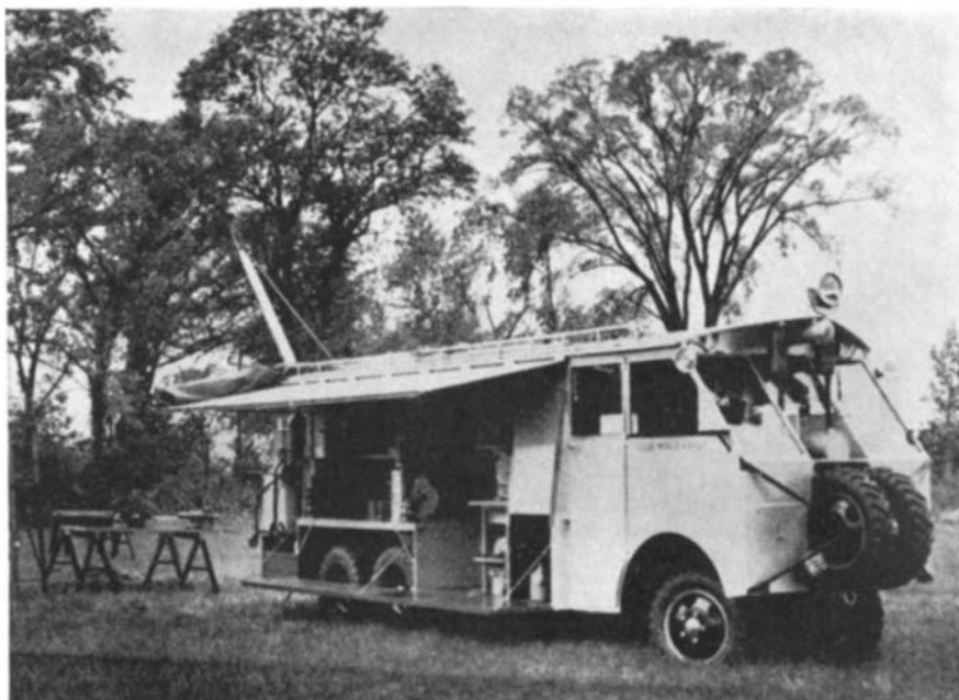
A mobile airport provides mechanical servicing facilities in the field
