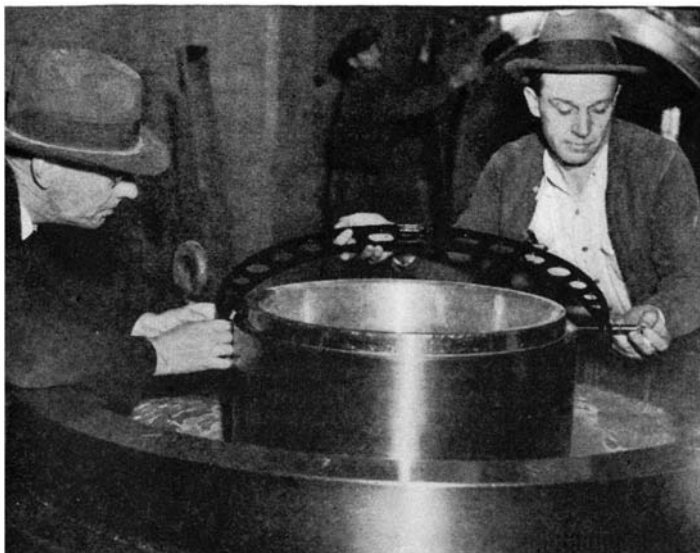
Below: Pump replacements and repairs will be difficult and expensive, so the greatest care is taken to insure proper running fit between bearing surfaces. Here two engineers are "miking up" one of the large bearing rings used in the pumps
