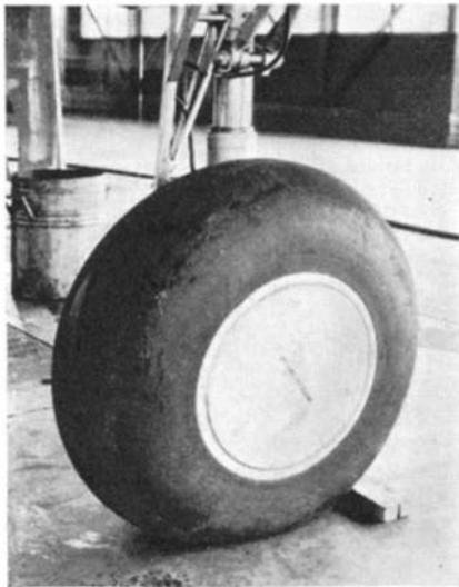
Above and left: Views of the improved streamlined airplane wheel
