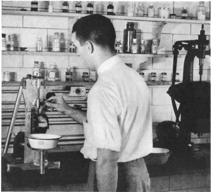
Froth flotation tests in the Bureau of Mines Laboratories. Research is continually under way in these laboratories to increase the recovered values of minerals
