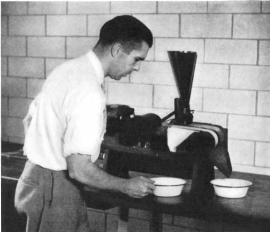
Developing a practical separation of minerals in a magnetic machine. Such research has resulted in large gains in conservation of our mineral resources
