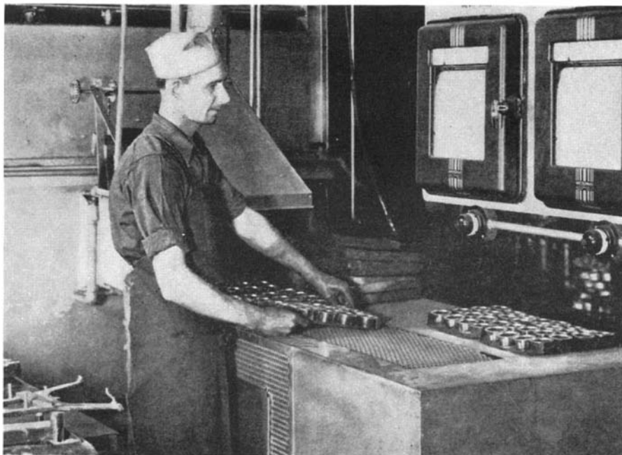
Pressed bearings, made as in picture above, are sintered to cause diffusion of constituents. Here, they pass through a high-temperature furnace on a conveyor
