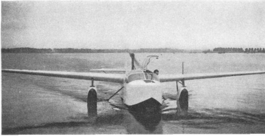
Above: The Spencer-Larsen amphibian. Below: Drawings showing how the stabilizing floats and landing wheels are combined and pivoted so the wheels may be retracted
