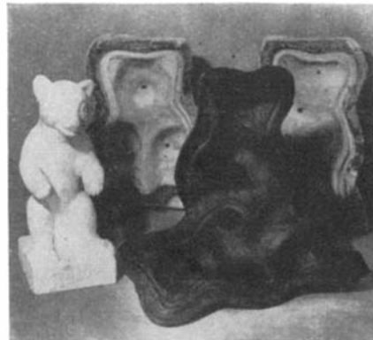
Molds of Korogel are pliable, can be removed from casting undercuts
