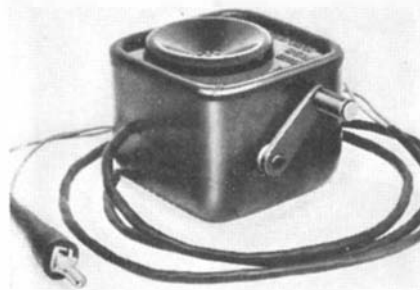
Voice-powered telephone that requires no battery. Hand crank is used only for calling the other party
