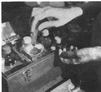
The solutions are filtered in the larger sets, in order to clarify colors
