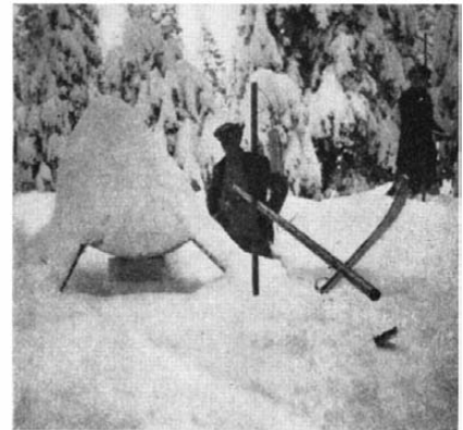
A snow pan protected from falling snow by a special covering or hood
