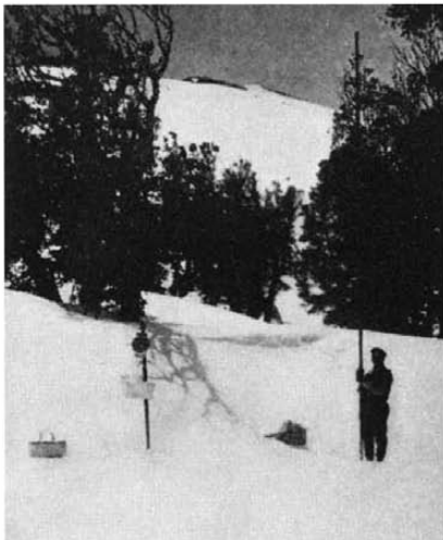
The height of the snow sampler in the man's hands shows snow depth
