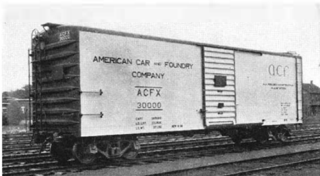
Two new types of freight cars constructed of light-weight alloys
