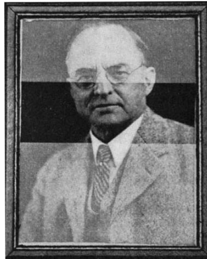
The clear part of this framed portrait is covered with the new invisible glass, the rest with ordinary glass to show the difference
