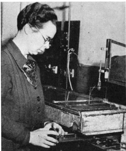
Dr. Blodgett demonstrating how the anti-glare surface is put on glass
