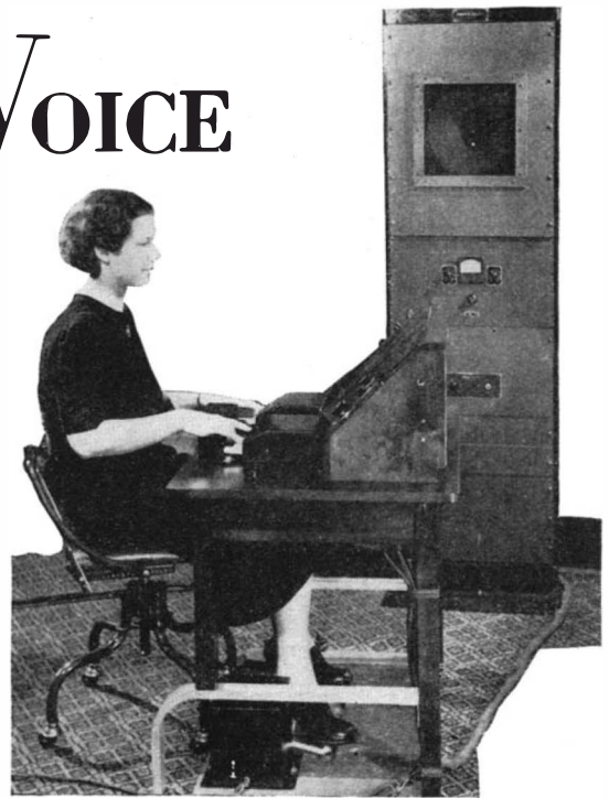
The Voder in operation. Foot pedal gives inflection to synthesized speech from loudspeaker
