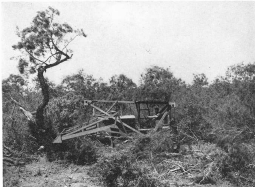
The "tree-dozer" showing, in small picture, the pusher bar and the heavier cutting edge beneath it. Below: The machine rips into large growth with no great effort
