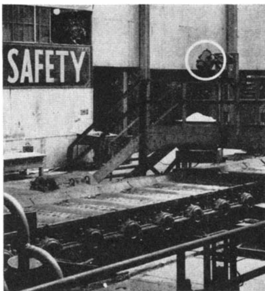
Above, in circle: Photronic photo cell mounted above a roll table in the strip mill at Fairfield Works of the Tennessee Coal, Iron, and Railroad Company. Right: A sample of slab-temperature record made by a Photronic pyrometer on a strip mill
