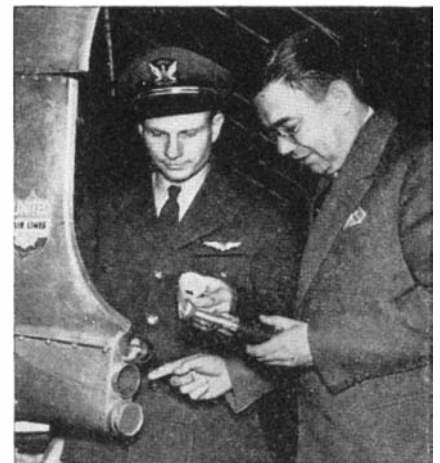
The static suppressor for airplanes is installed at rear of fuselage
