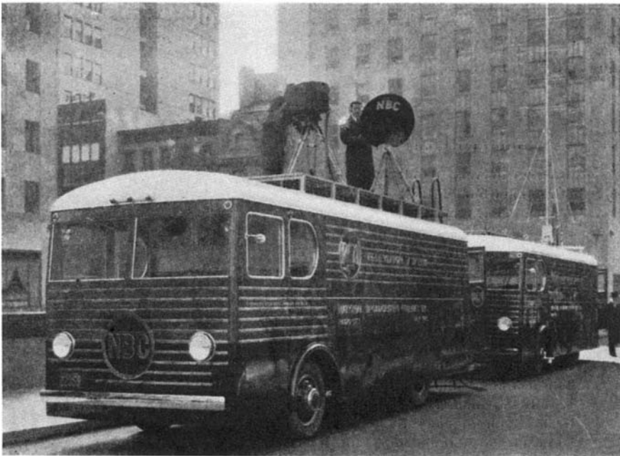
Mobile television unit consisting of two trucks that carry all equipment necessary for relaying television programs from remote points to the main transmitter located some miles away
