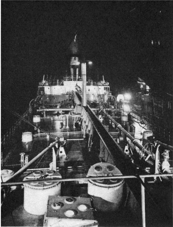
A modern oil tanker, the S. S. J. W. Van Dyke, at night. Note the well-protected passageway down the center of the deck
