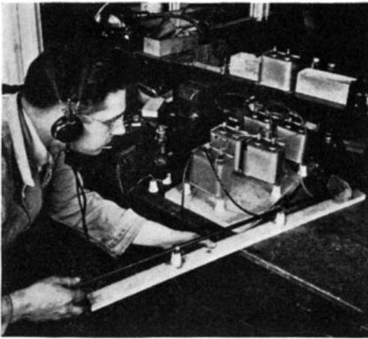
A laboratory set-up for creating man-made static for use in testing aircraft radio equipment
