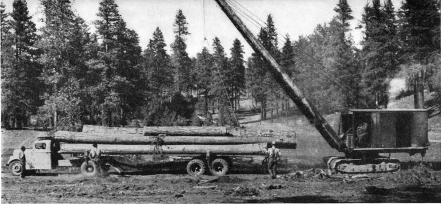
Loaded logging truck and Diesel converted shovel loader handling ponderosa pine logs in an Oregon forest
