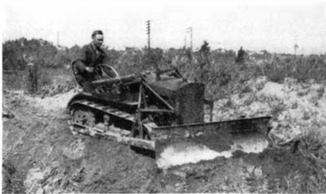
Less than three feet wide, this baby bulldozer-tractor builds trails in mountainous country that larger units may follow
