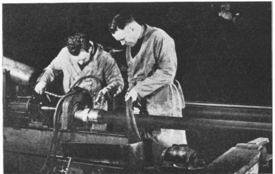
Left: The Tube-wall-scope in use. Below: With the Magnaflux test, invisible pipe defects are detected
