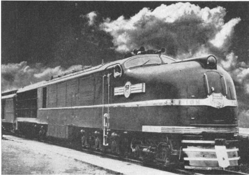
One of the two identical units of the new Union Pacific Steam-electric locomotive. Units may be operated separately or together. Note the engineer's high perch
