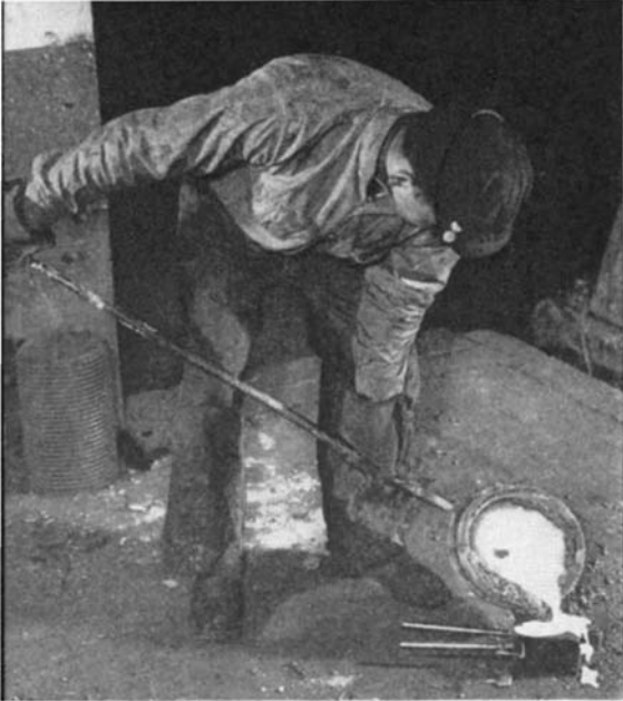
The first step in the process is the pouring of a sample from the molten metal into a hand mold
