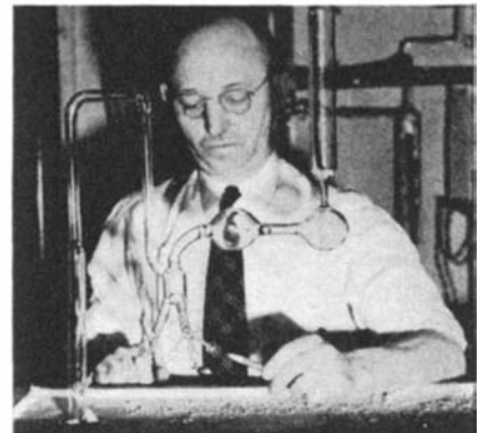
Above: One of the sodium bombs compared with the tube in which it will be used. Right: Final stage in the production of the bombs. Filled with triple distilled sodium, they are ready to be sealed and removed
