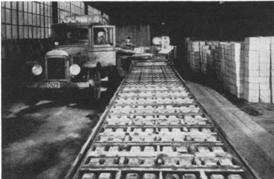
Above: Pouring the mix at one end of the continuous production Cemenstone mill. Right: A few of the pre-cast concrete shapes that can be produced with the same equipment
