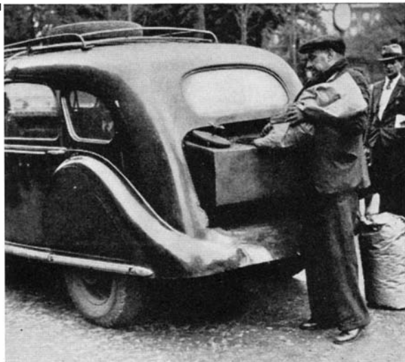
At right: A Parisian taxi driver attracts curious bystanders as he loads his wood-burning taxi with a charcoal-anthracite mixture. Below: Motorman's cab and wood-burning gas producer in a French passenger bus. At bottom of page: A German bus which carries compressed gas fuel in trailer tanks
