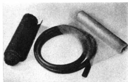
Koroseal: after processing, as extruded tubing, and in film form
