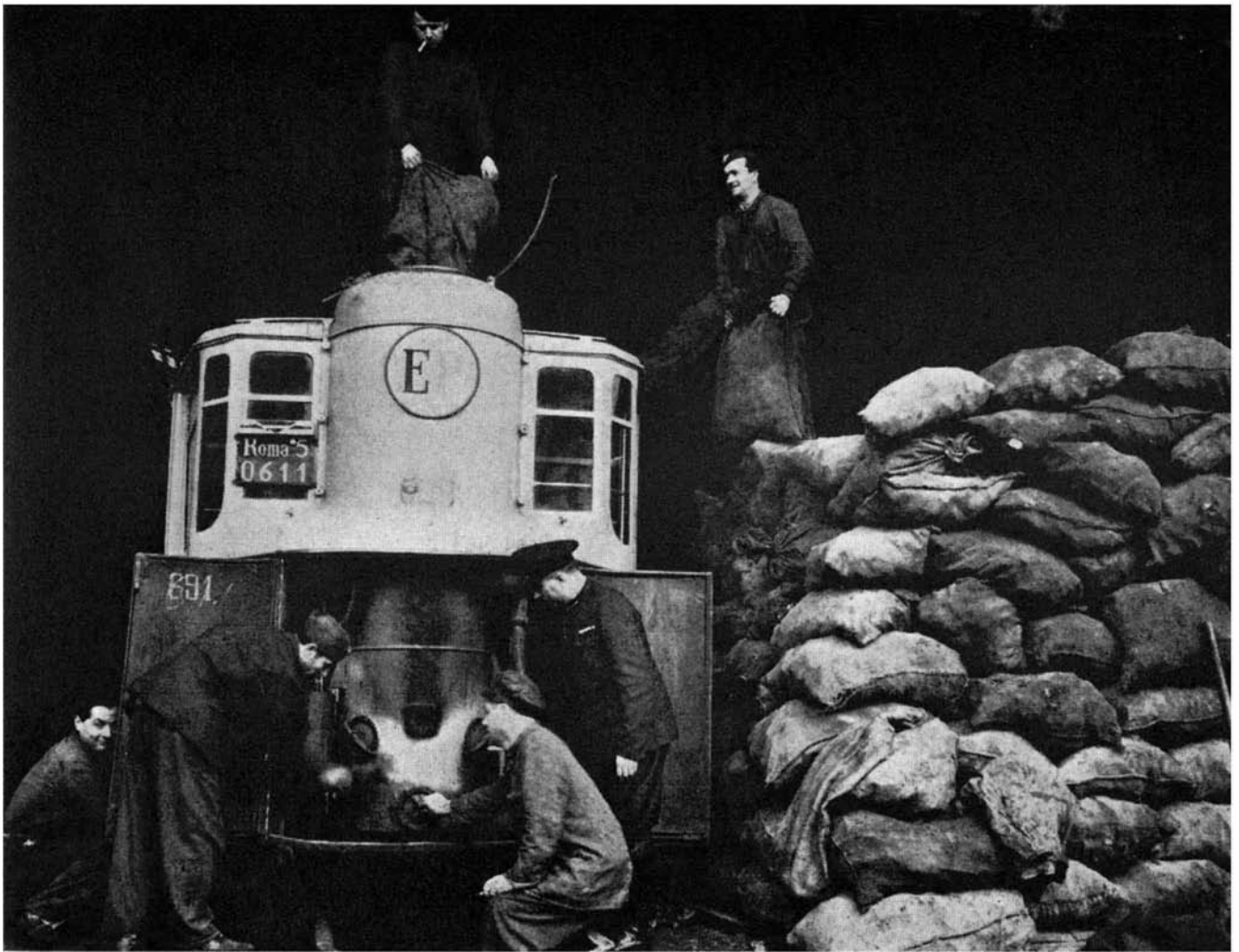
A strange sight to an American: a "filling station" for Rome's 85 wood-burning buses. Small furnaces, concealed in the rear of the buses, and charged with blocks of wood cut in small sizes (or coal or charcoal), generate the gas which the motor uses
