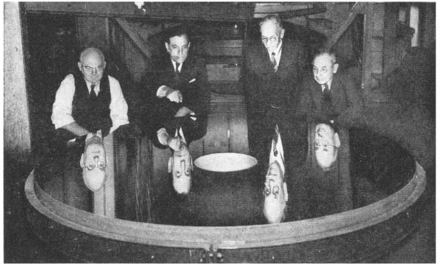
The 82-inch mirror, 12 inches thick, after aluminizing. From left to right: H. L. Cook, director of the Warner and Swasey Company's instrument department; C. A. Robert Lundin, director of the optical department, who figured the mirror; Dr. John S. Plaskett, director emeritus of the Dominion Astrophysical Observatory, who tested it; George A. Decker, works engineer. The focal ratio is f/4
