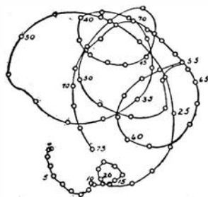
Map showing wanderings of an oil well, from surface (0) to full depth
