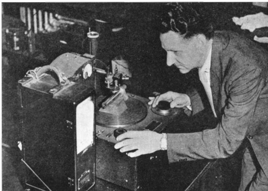
Objects to be tested for surface smoothness are placed on the turntable
