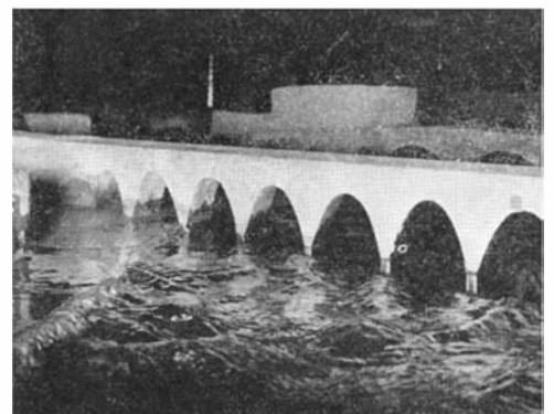
Above: Waves impinging on a model of a breakwater. Such waves as these must not enter the harbor
