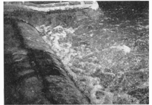
Model analysis of a spillway problem. The object of the engineers was to reduce water velocities and eliminate dangerous erosion below the dam. At the left, velocity was high and scour so bad as to cause much erosion. The model was then modified to produce lower velocity (right). Result was negligible erosion
