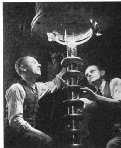
Lowering the 100-coil transformer over the tall and slender X-ray tube
