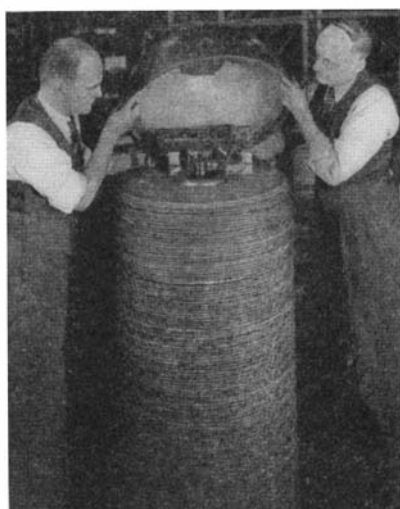
Revealing the filament end of the tube and part of control mechanism
