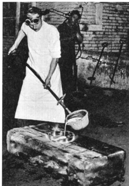
Above: Molten iron, poured on new glass chilled by ice, has no effect on it. Right: A 12-inch disk shrinks 1½ inches during processing. The glass is 96 percent silica
