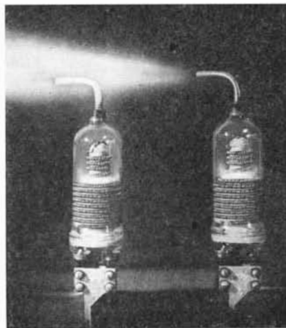
Midget electric boilers generate steam after 15 seconds of operation
