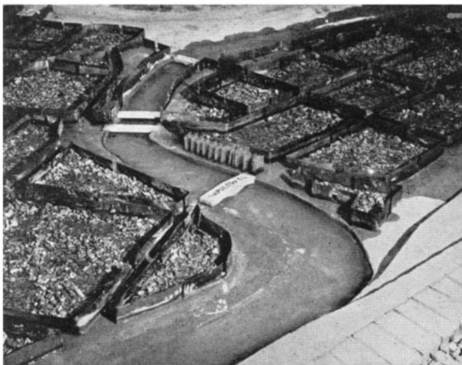
A model of the river through Johnstown, Pennsylvania, by means of which a very serious flood problem was solved
