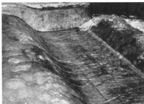
Model analysis of a spillway problem. The object of the engineers was to reduce water velocities and eliminate dangerous erosion below the dam. At the left, velocity was high and scour so bad as to cause much erosion. The model was then modified to produce lower velocity (right). Result was negligible erosion
