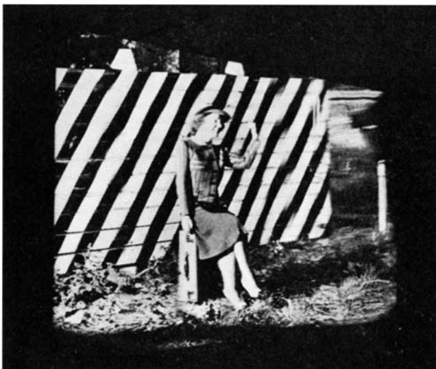
Distortion, caused by looking through safety sheet glass (left), and the clear view through safety plate glass
