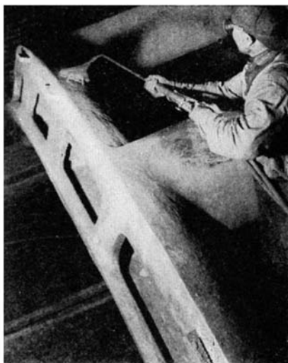
Flame-descaling a casting with a special oxy-acetylene heating head
