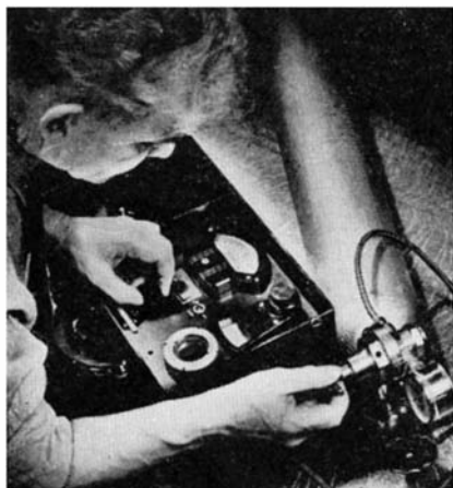
Dew point, and hence moisture content, of gas being read directly
