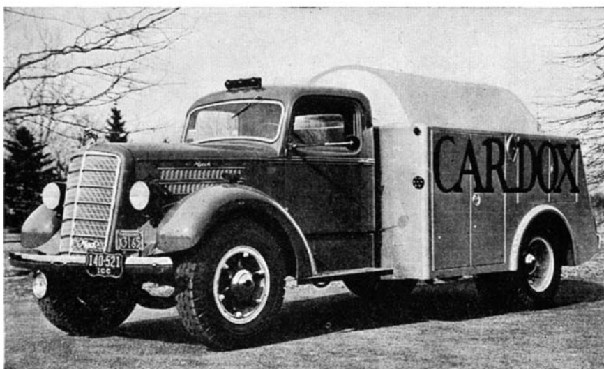
Insulated tank truck for transporting liquid CO 2 at constant pressure
