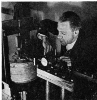
Above: Adjusting the "punching power" of the machine that tortures steel blades for steam turbines until they fracture as shown at left
