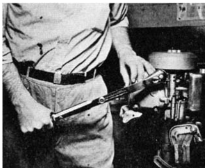
Uniform tension on series of bolts is possible with this new wrench
