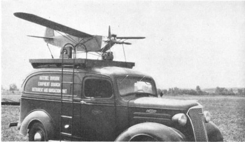
A truck is used for transporting the radio-controlled target plane to and from the anti-aircraft range
