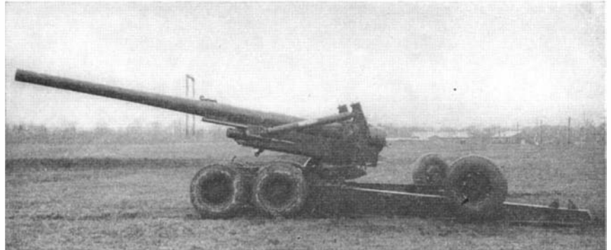
The field piece can be elevated to 65 degrees above the horizontal
