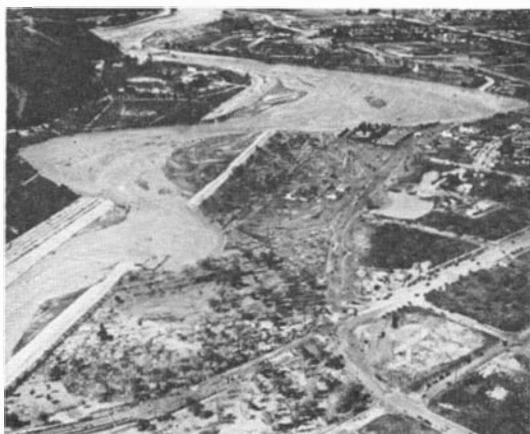
Los Angeles River during the flood of March 1938. Abrupt curves, where river breached and caused damage, have been straightened
