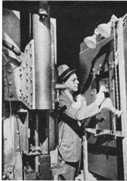
The pin-hole drum, carrying film of the high-speed camera, revolves behind opening at right center
