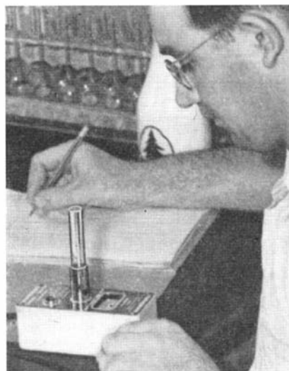
Milk undergoing phosphatase test
