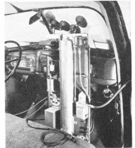
Car with anemometer and fifth wheel speedometer. The former determines wind direction, velocity; the latter gives an accurate speed reading. At right: Instruments within the car for use in conjunction with those shown above
