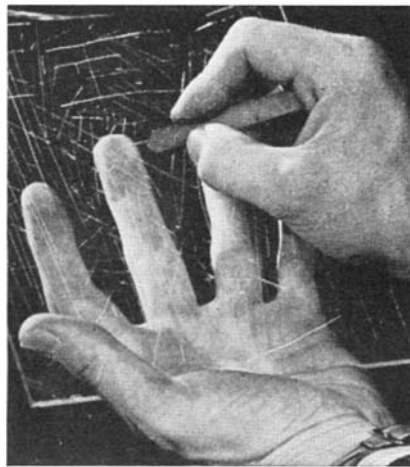
Air-hardened steel scratches glass, approaches the hardness of diamond
