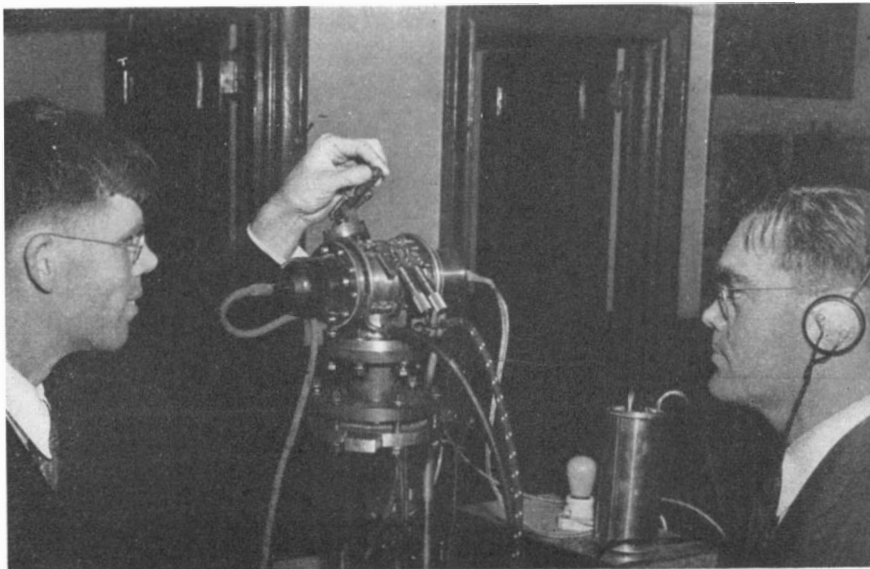
Russell H. Varian (left) and Prof. W. W. Hansen, conducting tests with one of the complete assemblies of two rhumbatrons sealed within an evacuated casing
