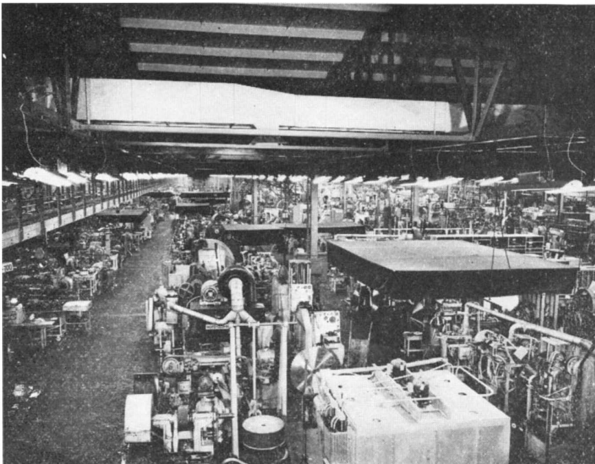
Eight self-contained production lines, each with a complete sequence of heat-treating to finishing facilities, function smoothly in the five-acre room
