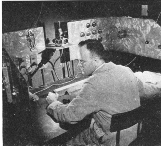
The control panels of the unique device which measures the lengthening effect of alternating current on magnetic metals, and developer S. L. Burgwin
