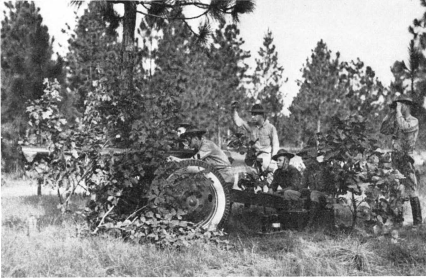
The gun, as modernized, is an excellent anti-tank weapon because its traverse of 90 degrees permits point-blank or distance fire over a wide fan-shaped area
