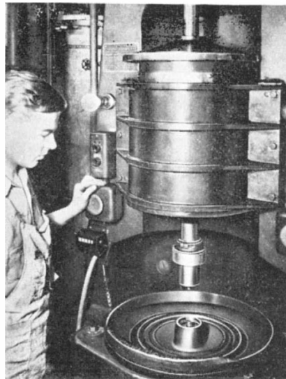
An automobile hub in the induction heat treatment machine described
