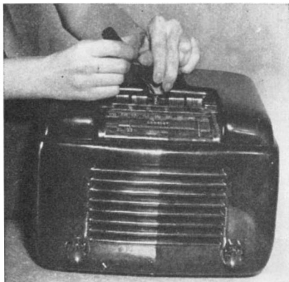
Lifting one of the flaps to re-tune a new push-button radio receiver
