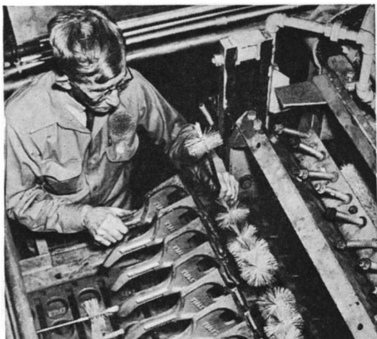
Durable and sanitary, nylon bristles are here being used to wash bottles, one of many uses
