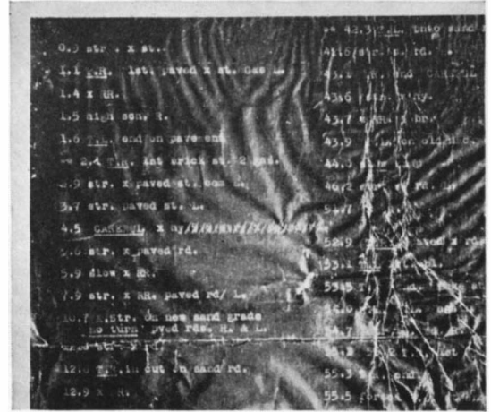
Section of a piece of carbon paper, photographed under slanting light, reveals message
