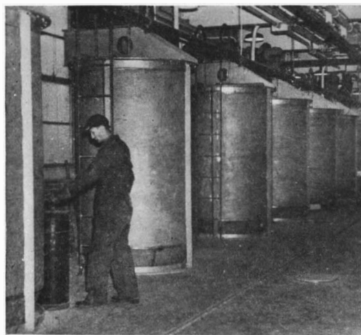
These "blenders" contain nylon chips about to be transformed into yarn for various textiles
