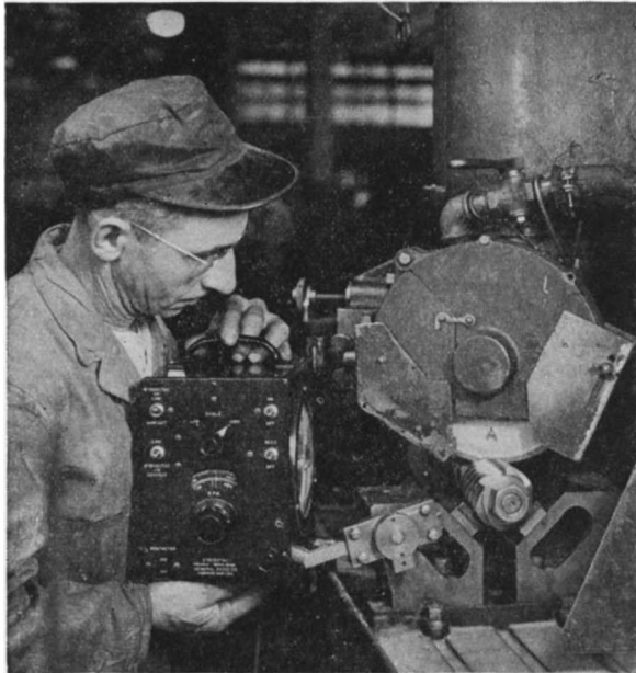
A portable stroboscope is used by the Boston Gear Works to watch gear-grinding angle and check speed
