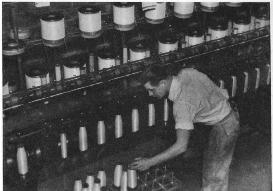
Nylon yarn being processed. Machines twist the bundle of slender filaments for ease in handling. Finished yarn consists of many fibers twisted into thread
