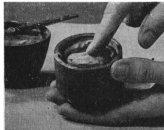
The wax pattern with painting completed, above, left, is placed, point down, in the casting flask above, center. The top of the flask ready for casting is shown at right, above. This is placed in a centrifugal casting machine, the platinum-palladium-gold alloy is melted with a gas and air torch in a cup before the sprued mold, and the machine is whirled to throw metal into all parts of the mold hollows left by melted wax.
