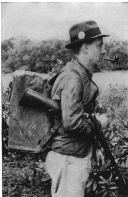
Above: Operating pump of portable water filter. Below: The entire unit may be carried on the back
