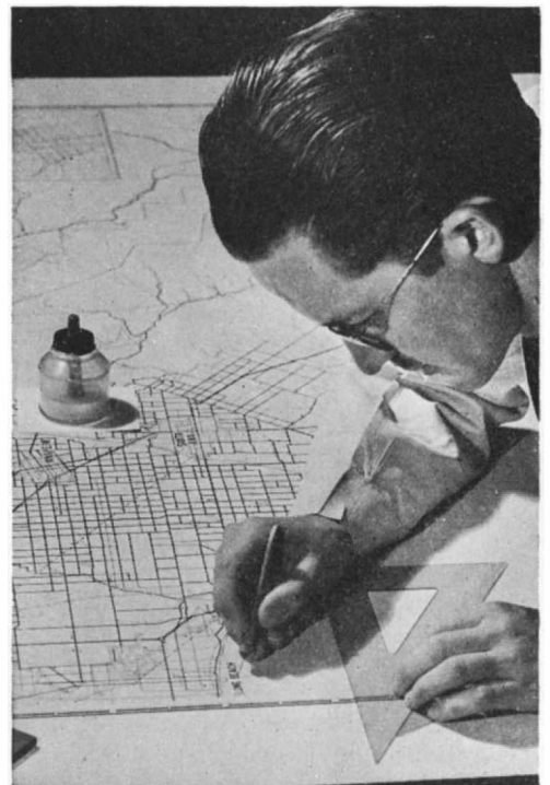
Preparing wet-plate negative from which lithograph plates are made
