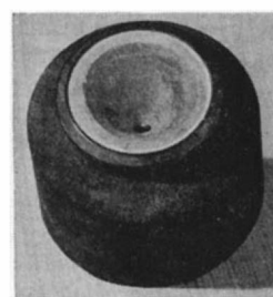
The wax pattern with painting completed, above, left, is placed, point down, in the casting flask above, center. The top of the flask ready for casting is shown at right, above. This is placed in a centrifugal casting machine, the platinum-palladium-gold alloy is melted with a gas and air torch in a cup before the sprued mold, and the machine is whirled to throw metal into all parts of the mold hollows left by melted wax.
