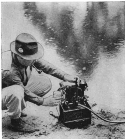
Above: Operating pump of portable water filter. Below: The entire unit may be carried on the back
