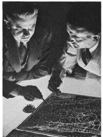
Preparing wet-plate negative from which lithograph plates are made
