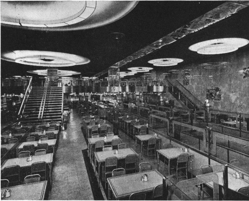
Overhead lighting fixtures at the left are semi-circular; the mirrored wall gives full-circle illusion. Structural flat glass, with sand-blasted designs, used at right
