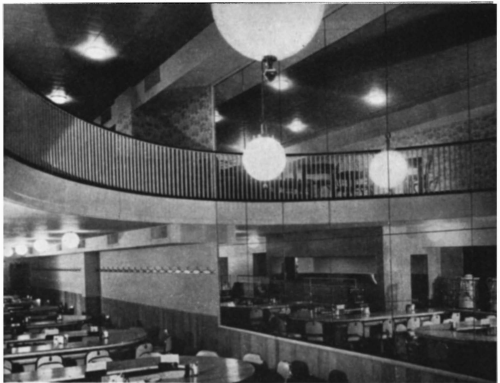
It is done with mirrors. The mezzanine rail is built against the mirrored wall, adding a touch of spaciousness and luxury to the surroundings that would be difficult to obtain in any other way
