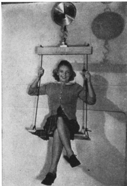
Magnet holds 4450 times own weight
