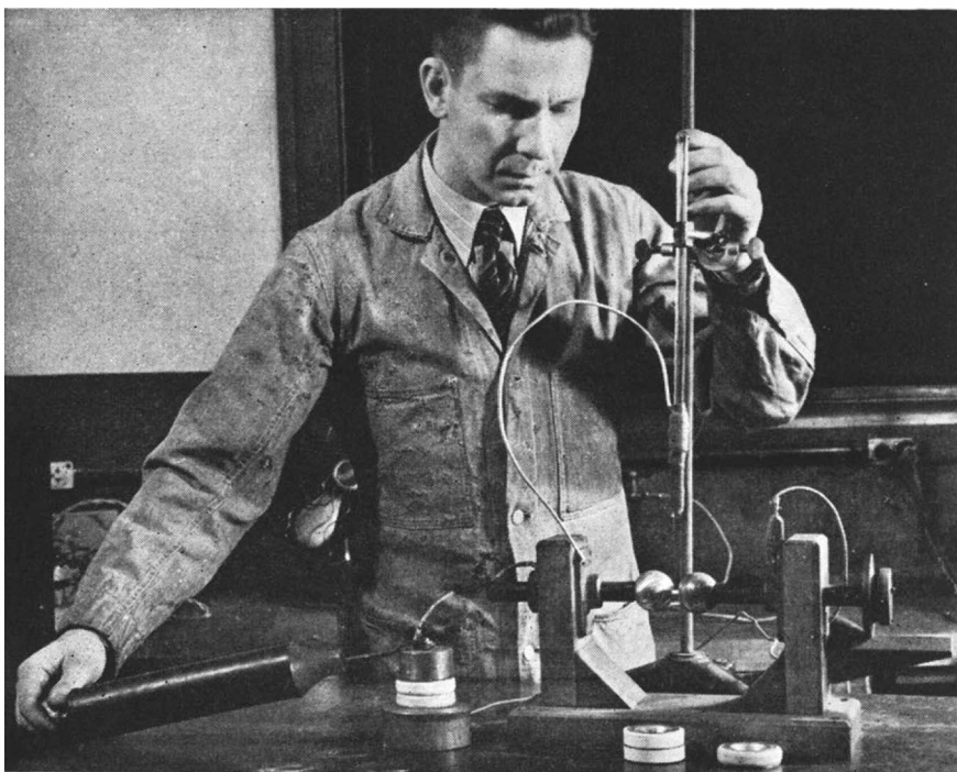
High-frequency radiation in the gap between the spheres makes the gap "fast"
