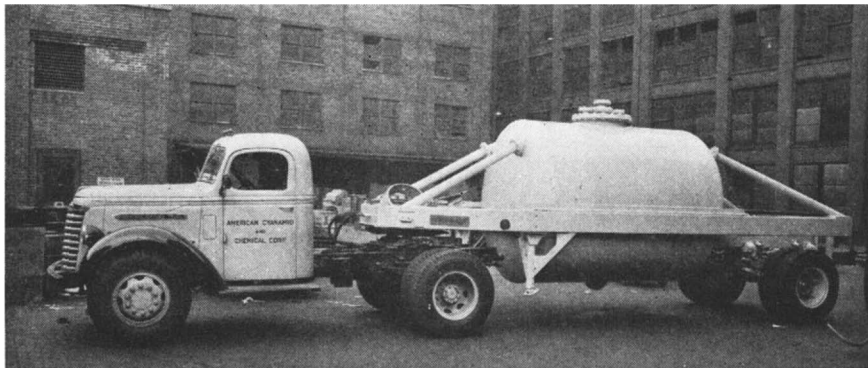
Two things — motor trucks and the relatively new process of adhering rubber to metal — provide the modern means of transporting large quantities of chemicals shown here. This special trailer tank of 2500 gallon capacity is lined with rubber so that it will carry corrosive solutions. It is one of two such trucks put in service by the American Cyanamid and Chemical Corporation; the tanks were lined by the Goodyear Vulcalock process
