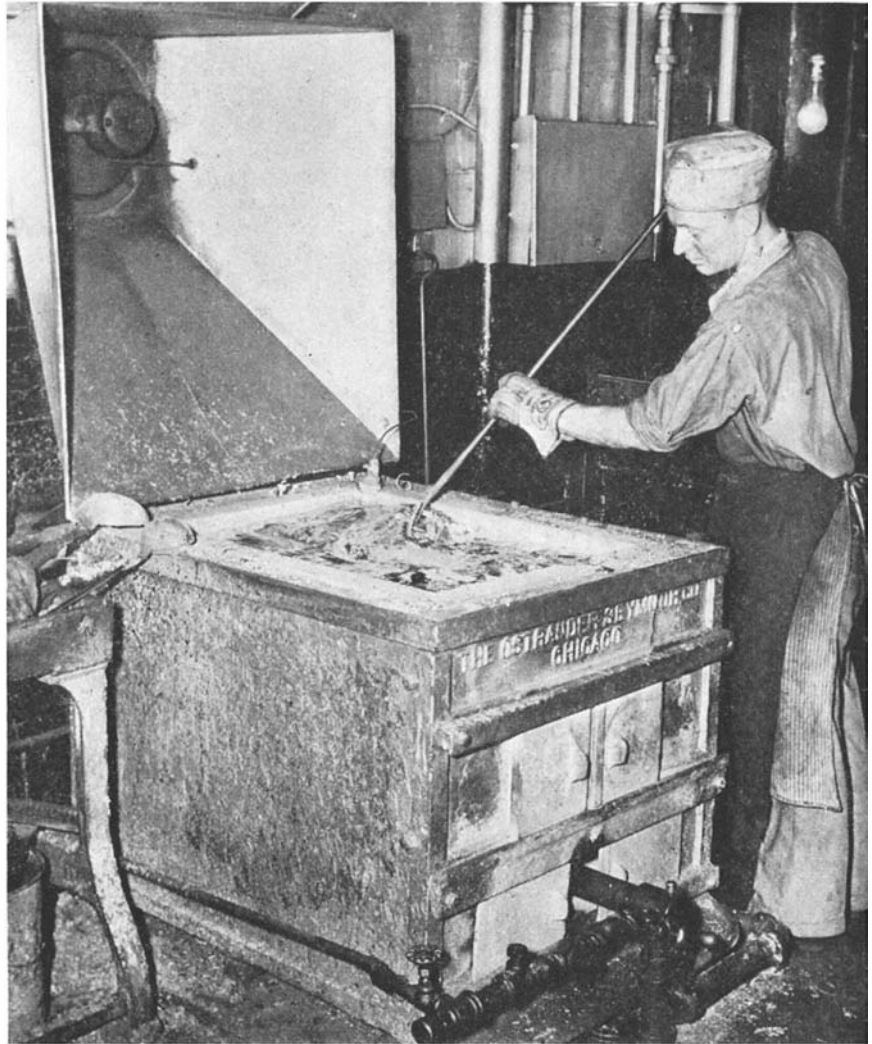
Fumes from molten lead can be a cumulative, slow poison. The workman shown here is safeguarded by the powerful ventilator at rear which draws off fumes
