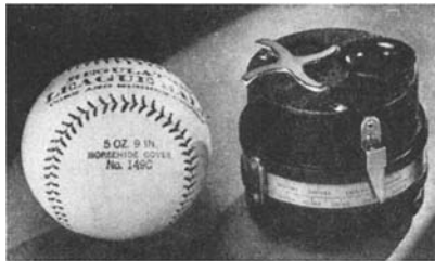
Self-powered stroboscope compared with baseball for size. Upper right: The instrument in operation
