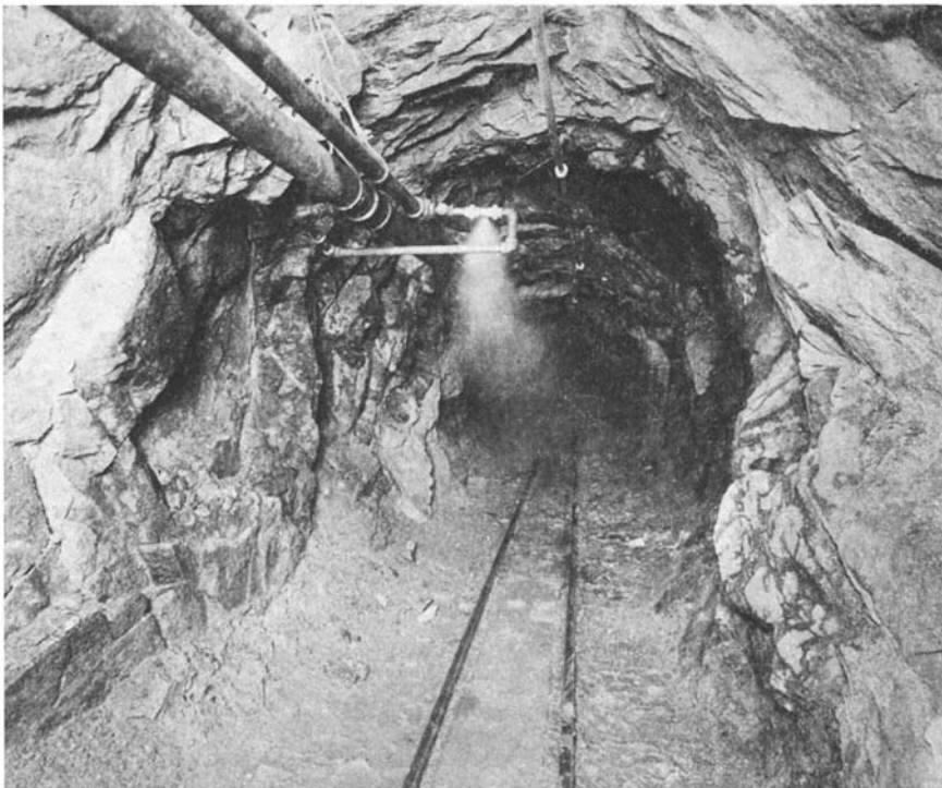
Compressed air-water atomizing spray used for humidifying mine air. This Laird type spray is also used to eliminate dust and gases caused by blasting
