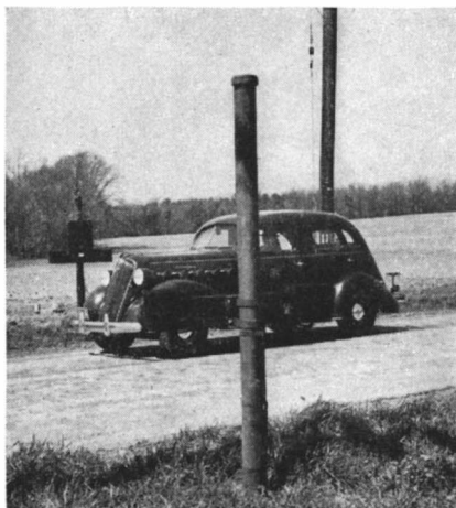
Permanent automatic traffic counter installed on a road in Maryland
