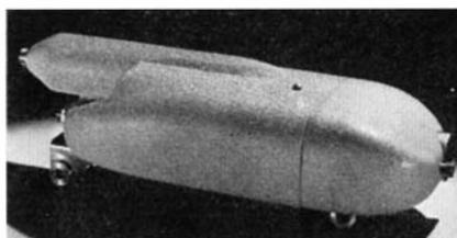
Above: Fixed type camera gun, and, below, cameras (in circles) mounted on upper plane wings
