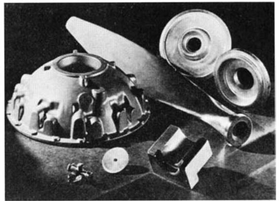
Below: Extruding an alloy of magnesium. It can also be die cast, sand cast, forged, and welded. At right: Airplane propeller blade and other aviation parts made of Dowmetal, world's lightest, strong structural metal
