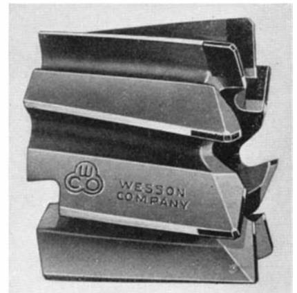
Bonded edges of cemented carbide in a standard tool
