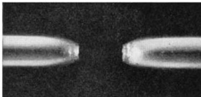
Ductility and smoothness of PDCP shown by rupture test
