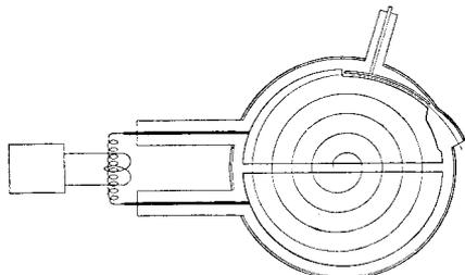
Plan showing main elements of a cyclotron's vacuum chamber
