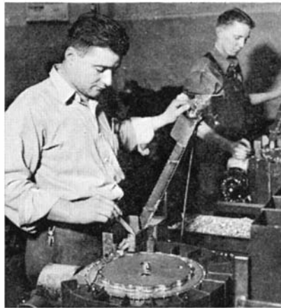
Steps in salvaging rivets. Lower left: Sorting for diameter with sifter. Above: Sorting for length. Below: Separating round-heads from flat-heads
