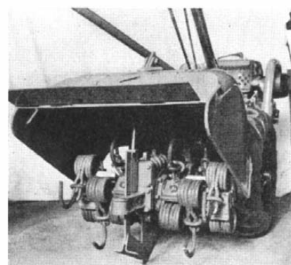
Left: Shredding garden soil with the motorized tiller. Above: Rotating tines that do the work
