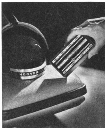
When determining the speed of rotating parts with a new tachometer, it is only necessary to hold the tachometer case in contact with machine housing
