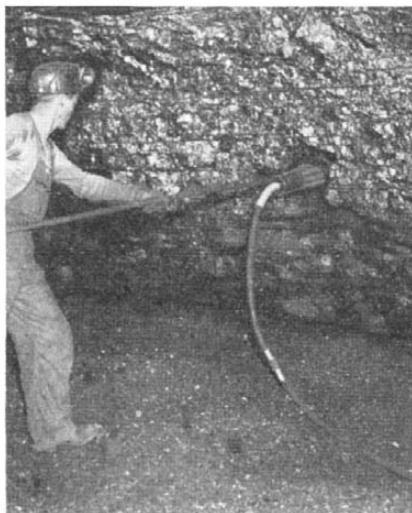
Inserting a hydraulic mining tube in face of a coal vein
