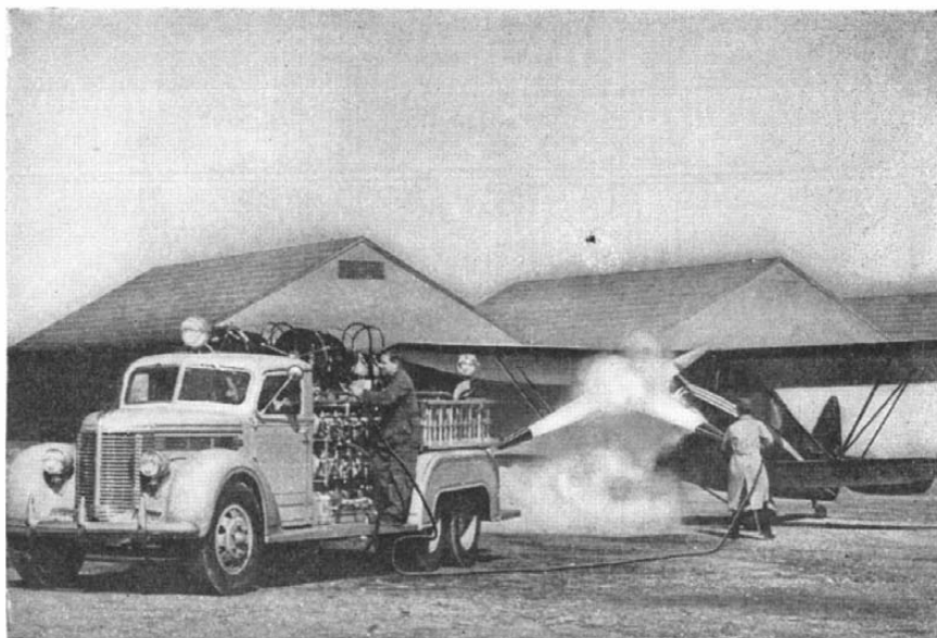
Above: Airport fire-fighting truck that carries 1000 pounds of compressed carbon-dioxide gas as well as grappling hooks and a derrick. Left: A motorcycle unit used by the Navy. Right: A small trailer unit carrying 150 pounds of the gas
