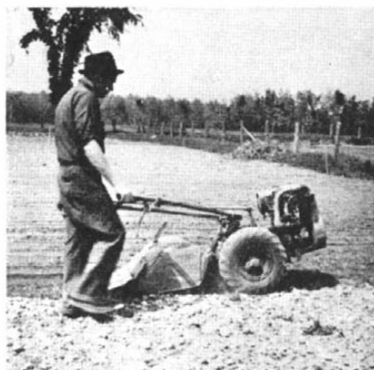
Left: Shredding garden soil with the motorized tiller. Above: Rotating tines that do the work
