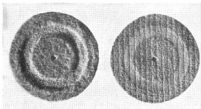
Above: Compact cloth tester in use. Below: Typical cloth sections after test, showing how surface is worn by the Abraser
