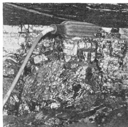
Close-up of the mining tube that expands under pressure
