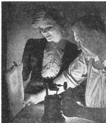
Testing fire-retardant insulation under blast of blow torch
