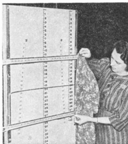
A garment is measured before the cleaning, and it must go through the process without any shrinking or stretching or alteration of original shape
