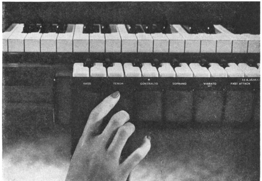
Above: The Solovox, a musical supplement to the piano, has a six-octave range and an indefinite variety of tone colors. Below: Solovox keyboard
