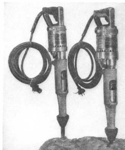
Representative models of the electric hammer described here. The hammer-holding chuck can be seen through the case hole
