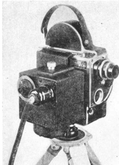
Above: Bolex camera with Synchronsound drive. Below: Turntable unit, five-minute disks
