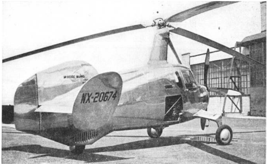
Above: The PA-36 autogiro, showing engine compartment with cover removed. Below: Line shows vertical take-off
