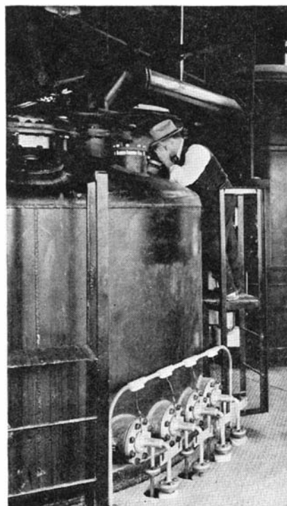
Peep holes enable operators to observe first stage of process
