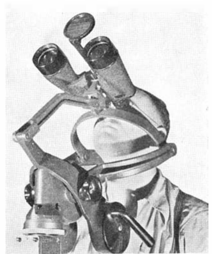
An airplane finder used in conjunction with powerful lights
