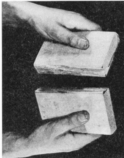
Rock maple, joined with cold-set glue, broke; the joint held
