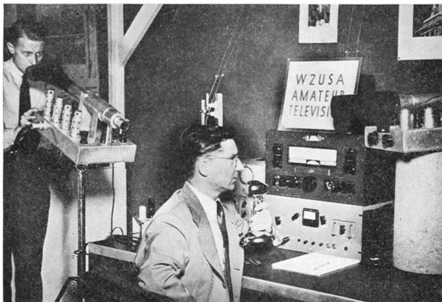
Two-way amateur television set-up. Camera at left, receiver tube at right
