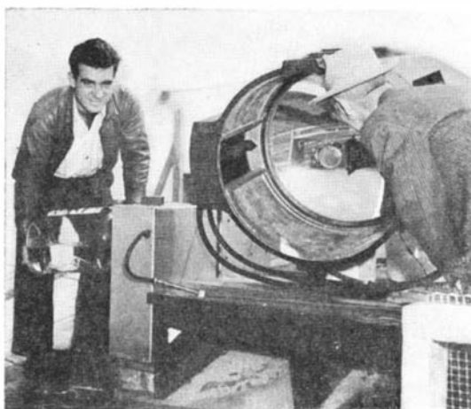
Water-cooled 24-inch "sunspot" lamp used to illuminate finish line for photo finishes
