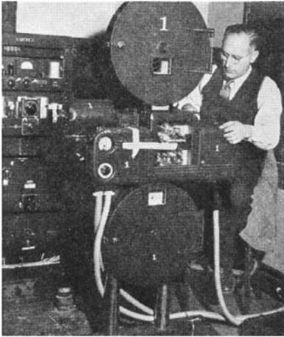
The projectionist inspects one of the special sound units in which is run the "Fantasia" film with its three sound tracks and the single control track
