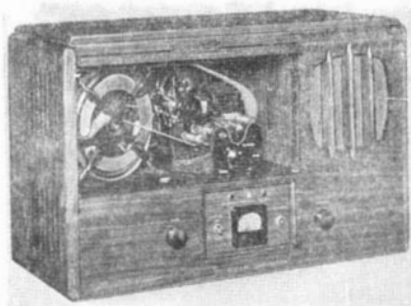
Panel of Recordgraph is lifted to show the interior mechanism
