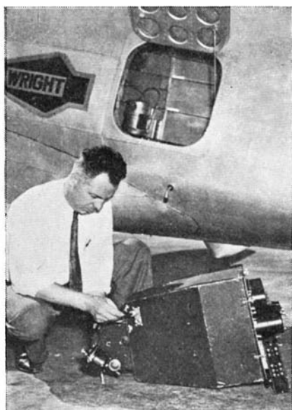
Preparing flight observer for installation in rear cockpit of two-seater military airplane
