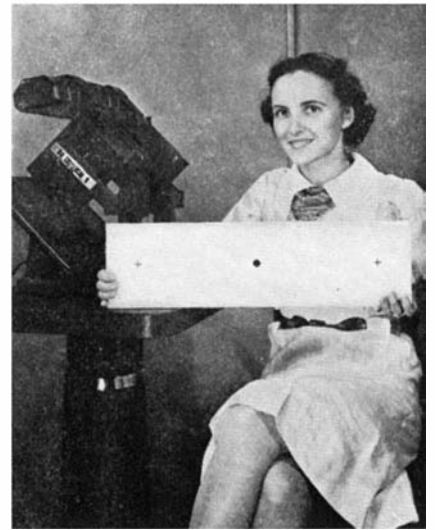
The stereo campimeter, at left, is used to measure blind spots, while the chart is a simple test to show up blind spots
