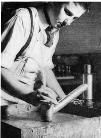
A crystal is ground to the correct angle, ready for finishing
