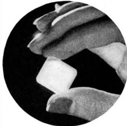
Finished crystal, ready for its mounting in which it will control accurately the frequency of a radio broadcasting station
