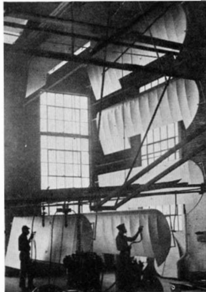
Wing-spraying "Ferris" wheel
