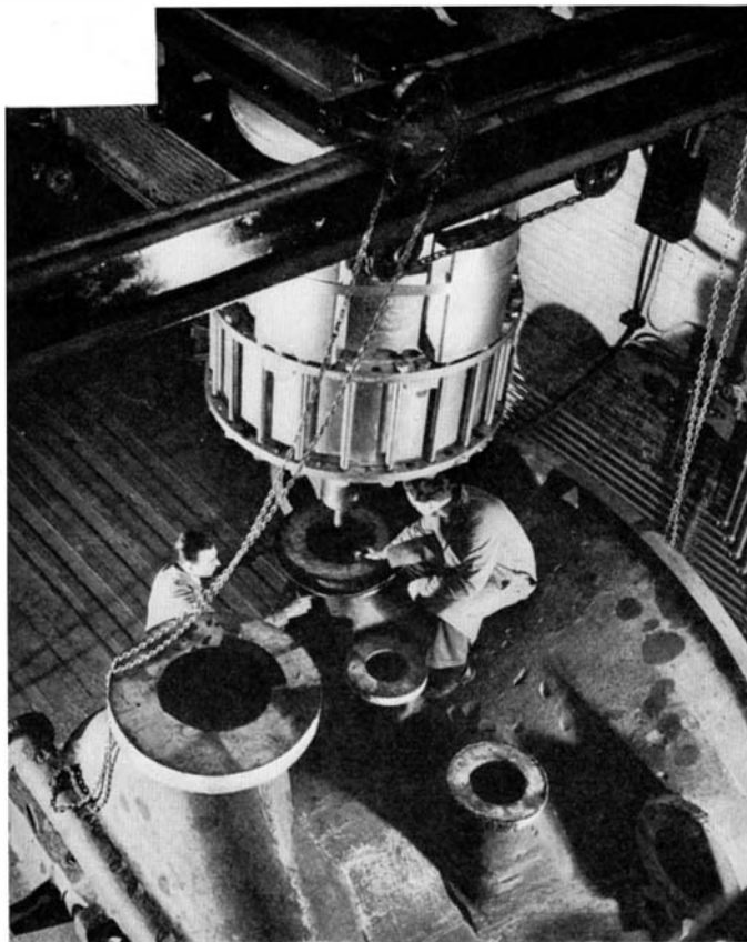
Business end of the 1,000,000 volt industrial X-ray unit being lowered into a huge steel casting to be studied
