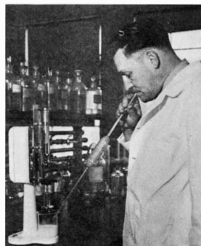
The curdometer for measuring the degree of softness of milk curds like those in the stomach
