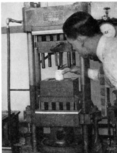
Melamine plastic drinking glasses being molded in small press
