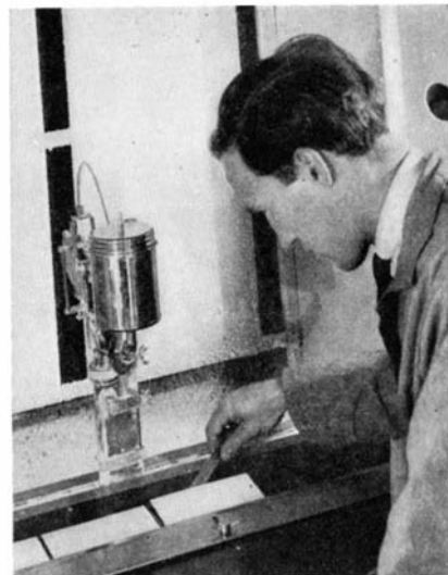
Test panels are automatically sprayed with melamine enamel
