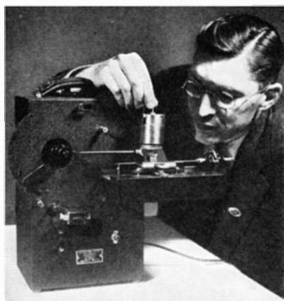
Power-driven sewing needle acts as human finger nail in tests
