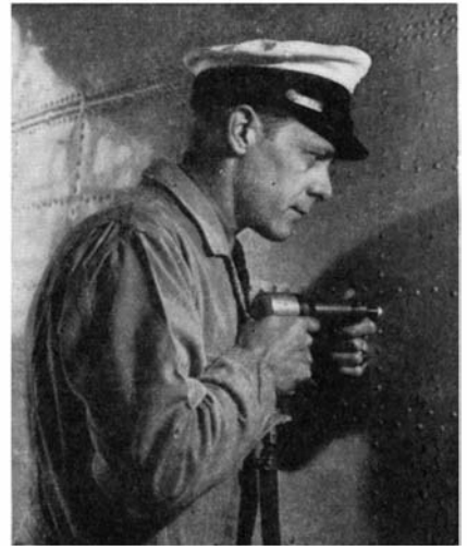
Like the Army, Pan American checks fuselage for loose rivets
