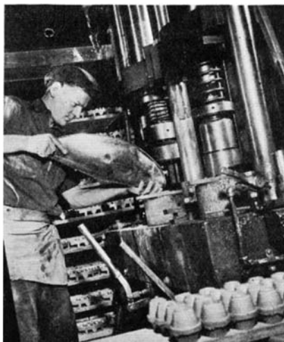
Pouring the dampened Prestite mixture into the forming die
