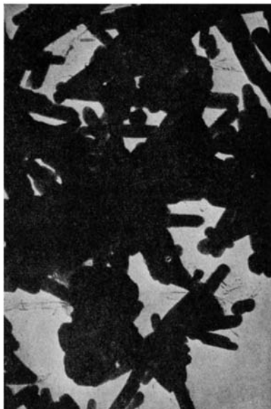
Electron micrograph at left (approximately 18,000x) shows calcium carbonate to be made up of tiny, elongated crystalline prisms. Compare definition with photo (right), made with light microscope, about 1000x
