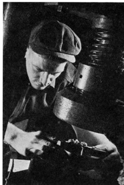
High pressure is used in this hydraulic press in which the damp clay mixture is formed into high-strength non-porous insulators for a wide range of applications in electrical work
