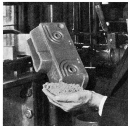
A handful of clay used in making the new electrical insulating material, as described on this page, and a formed fuse box
