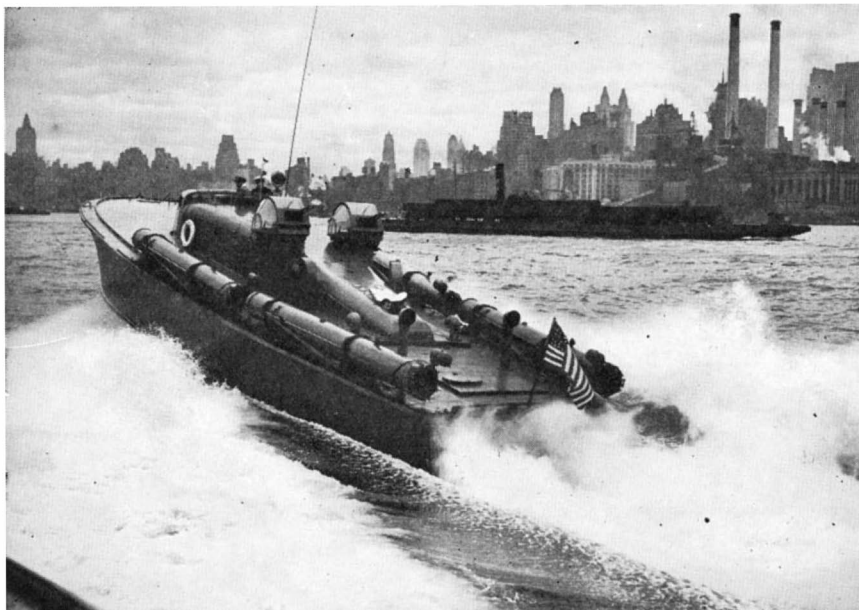
American motor torpedo boat, showing torpedoes, machine-gun turrets
