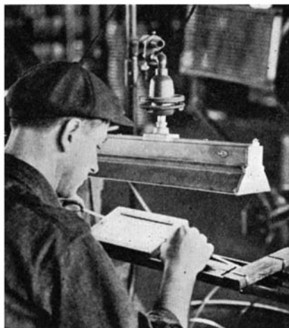
Fluorescent lighting fixture for inspection of metal strip. Inspector sees both sides of strip by use of the mirror shown
