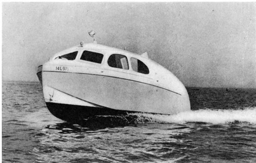
Plywood speed ship on trial run, Long Island Sound
