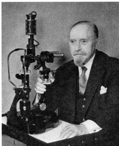
Dr. Max Poser with the instrument, combining a new slit-lamp and a wide-field binocular microscope, used in diagnosing a wide variety of eye diseases
