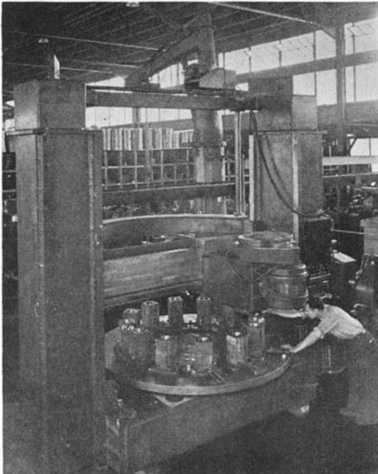
Arc welding reduced weight of this boring mill 15 percent; cut costs about 40 percent
