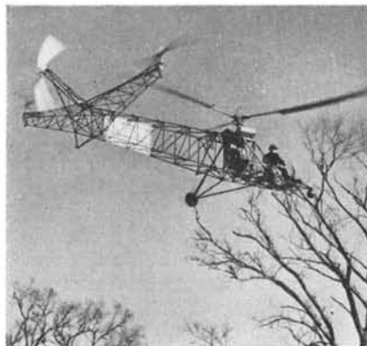
Hovering aloft near the tree tops, Mr. Sikorsky demonstrates complete control over his single screw, 90-horsepower helicopter
