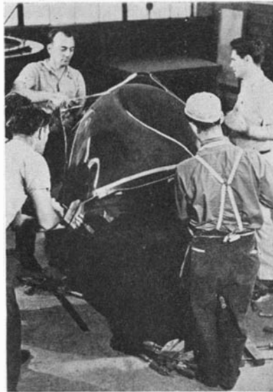
Left: The formed plastic sheet is cut with a band-saw to exact size. The material is shatterproof but is not actually bullet-proof
