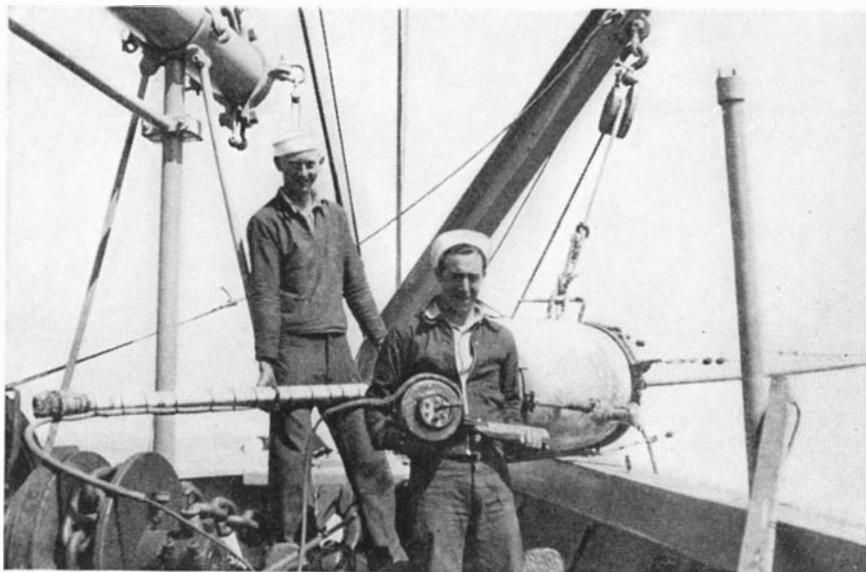
Figure 2: An all-metal sono-radio buoy (compare with sketch in Figure 1) and its attached hydrophone, in the arm of the sailor on right
