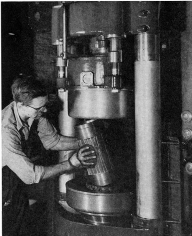
Placing a Diesel cylinder sleeve in position in the induction heat-treating unit for hardening operation
