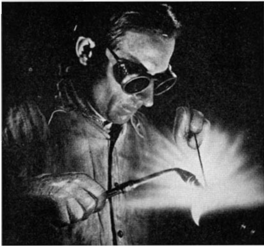
Absorptive lenses protect the welder's eyes
