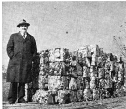
Used cans crushed and baled for shipment to a de-tinning plant
