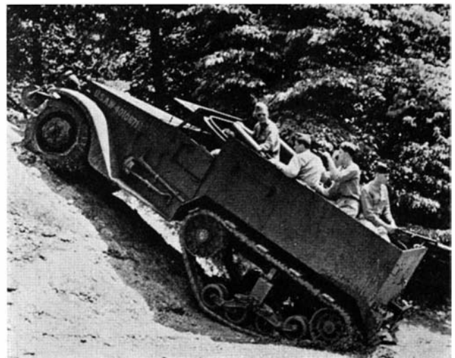
Chassis of the scout car described on this page. This type, manufactured by The White Motor Company, is powered by an engine developing 147 brake-horsepower. Right: A bank-climbing test
