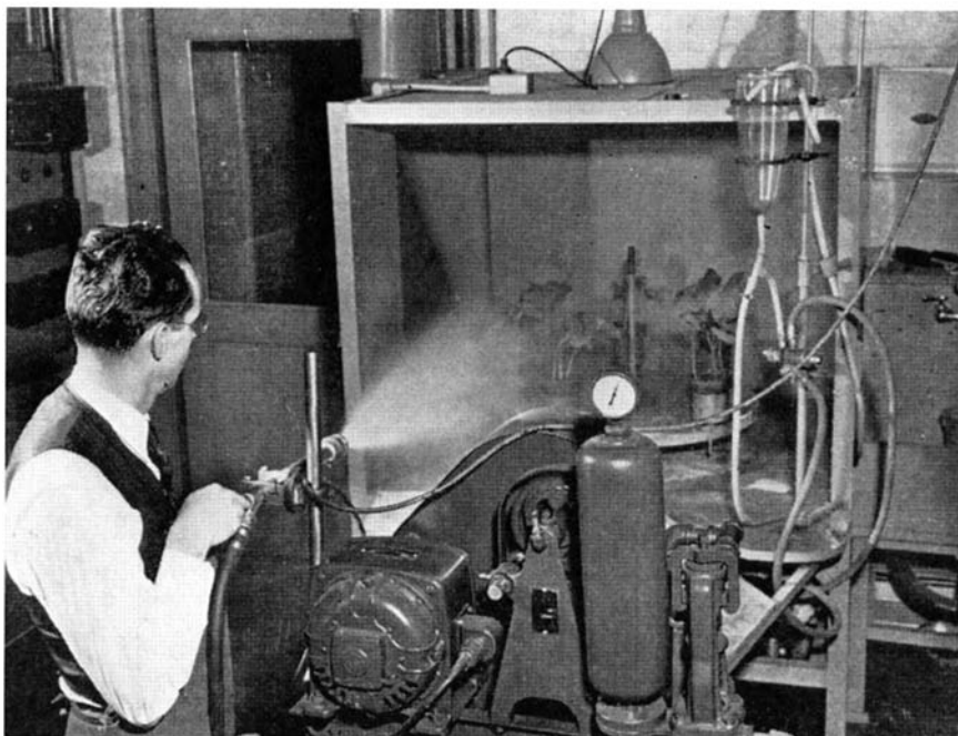
Laboratory apparatus duplicates effect of pressure sprayers used in field
