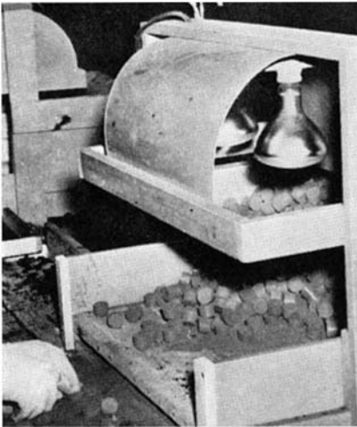
Removing moisture from pre-formed plastic before molding
