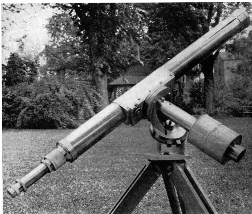
Figure 4: Taylor's 100-pound refractor with 3" triplet lens
