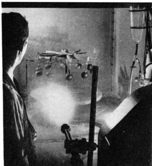
Apples are thoroughly coated with chemical spray in this laboratory setup. Codling moths are then hatched on the apples and spray value is checked
