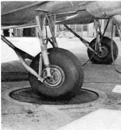
Wheel of a transport plane on the round iron saucer of the turntable
