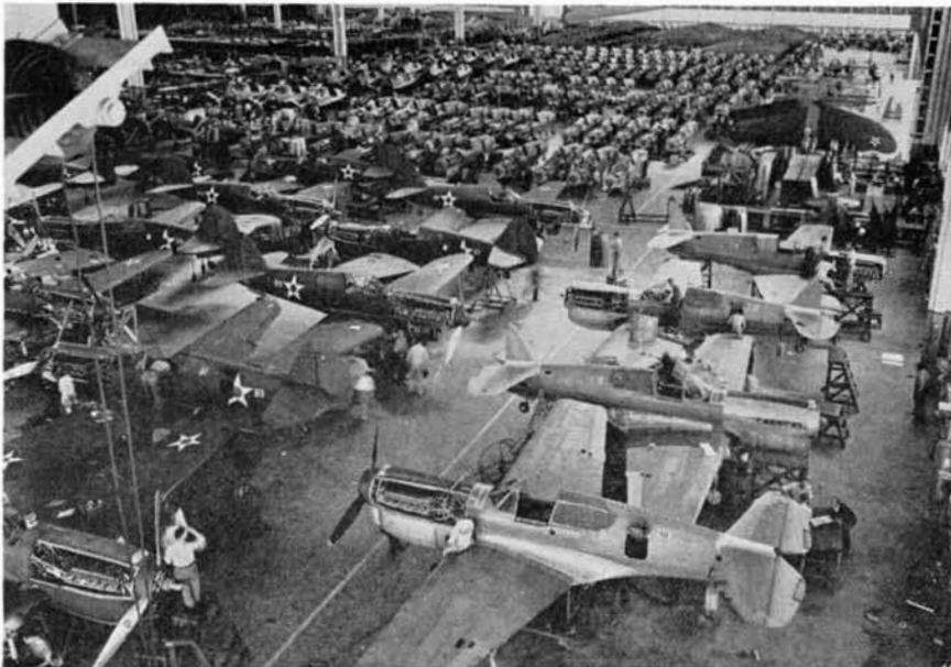
Final assembly section for Curtiss Hawks and Kittyhawks
