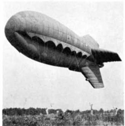
Small balloon, showing catenary curtain and the attached bridge
