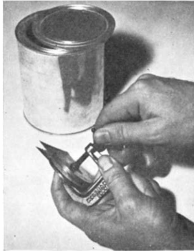
Above: Clamping film on both sides of steel disk. Below: Light areas indicate phosphorus
