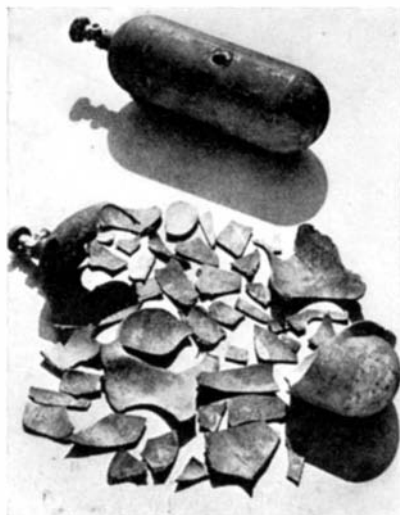
Above: One that can't burst and one that did. Right: Testing containers with .50-caliber armor-piercing ammunition
