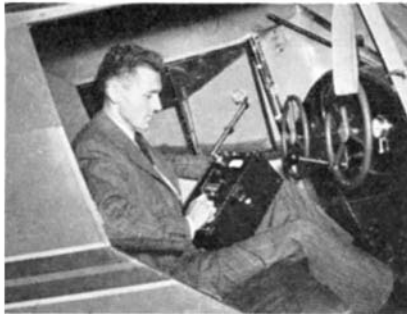
Measuring airplane noise level
