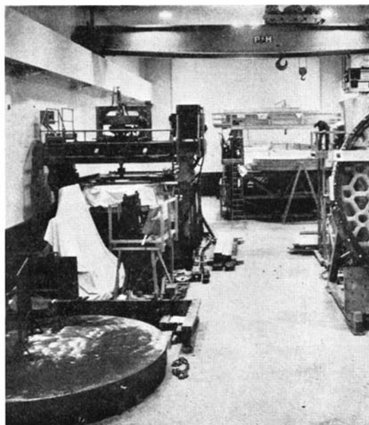
Figure 4: Five-ton, full-sized steel tool. Grinding and polishing machine in rear
