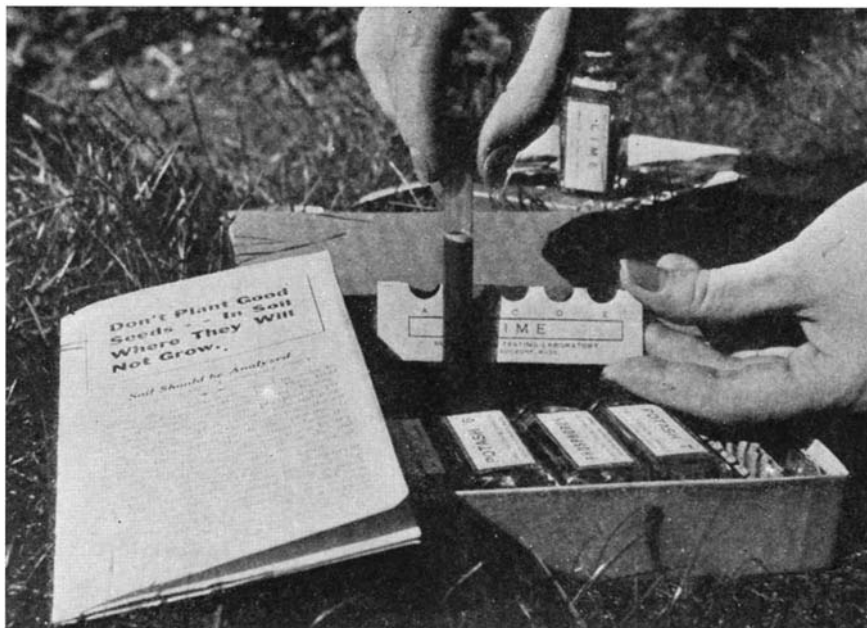
Solution of soil and reagent, in test tube, is checked with color chart
