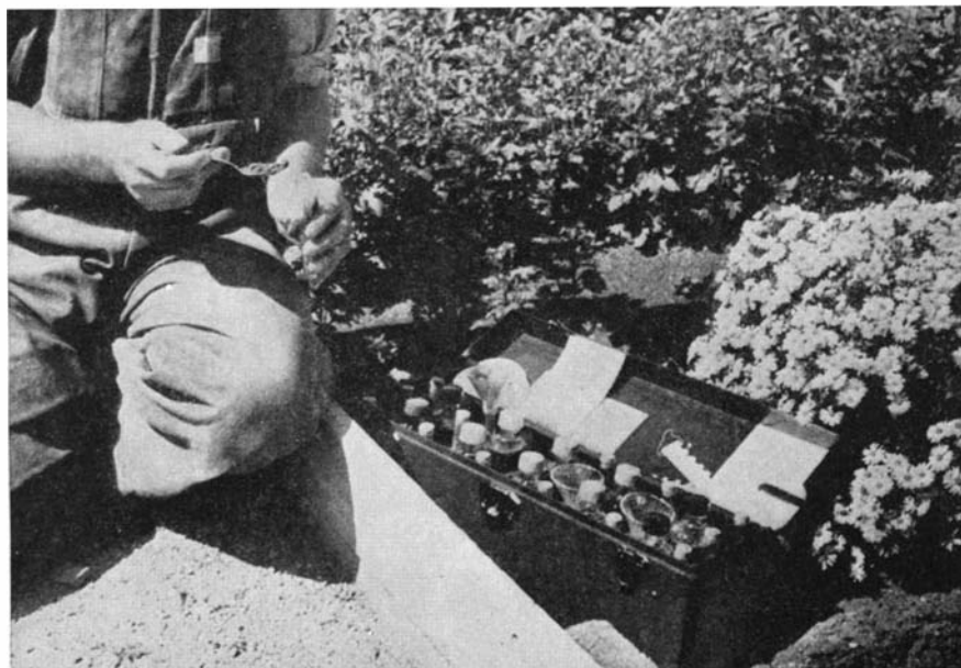
Soil sample is placed in test tube: testing kit with reagents at right
