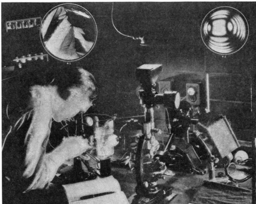
Petrographic microscope. Left insert: Crystal of organic compound. Right: Optical picture created in microscope by polarized light through crystal
