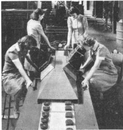
X-rays detect out-of-line washers
