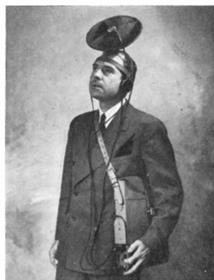
Microphone in headpiece, vacuum-tube amplifier in case at side
