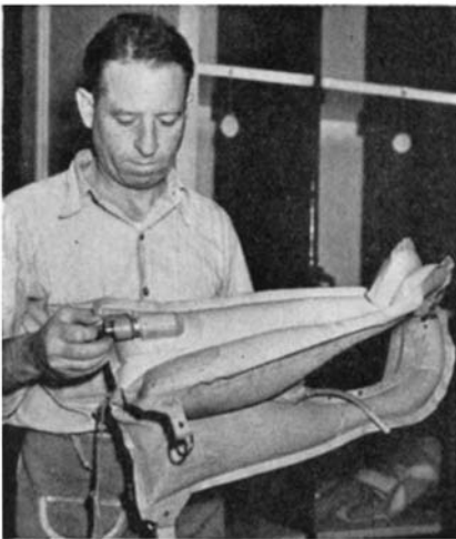
A small cylinder of carbon dioxide supplies buoyancy for life vest
