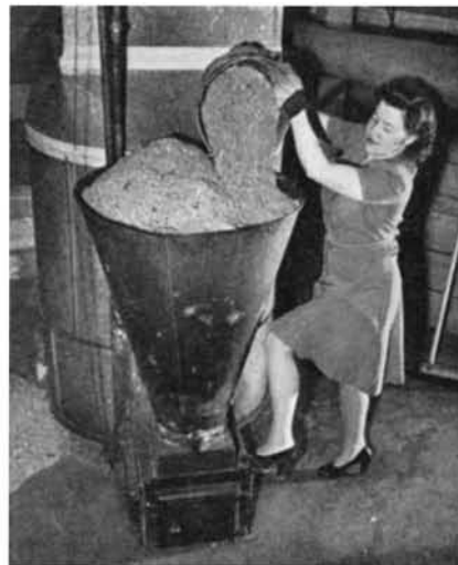
Hopper-fed sawdust burner
