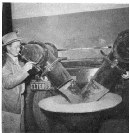
The fine cement is fed by screws to a cone, from which it is drawn to the slurry box for water mixing
