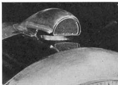
Above: Air scoop. Below: An ice-blocked carburetor intake system
