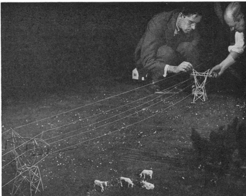
Building a miniature transmission line for studying lightning effects
