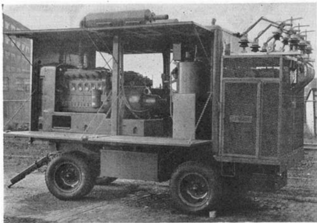
Two Diesels operate this mobile power plant
