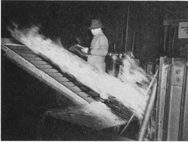
Left: Wind-blown flames melt asphalt, do not set roof deck aflame. Right: Firebrand test
