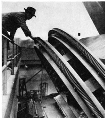
Figure 1: Worm wheel of 200"
