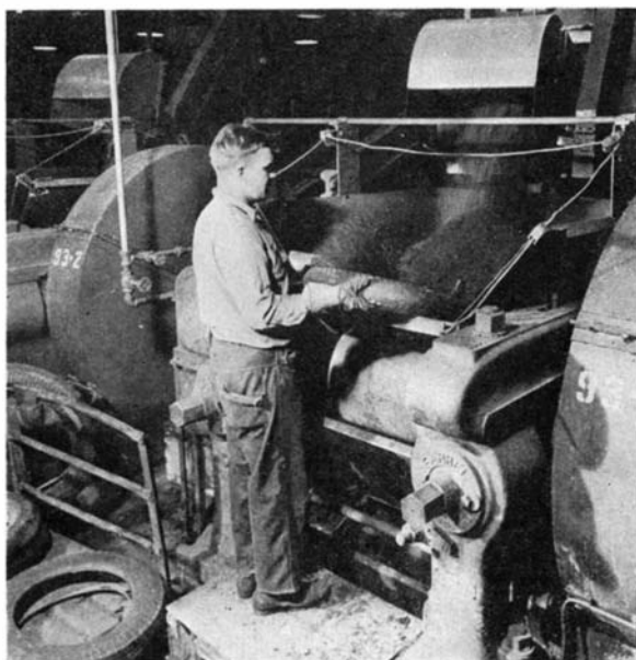
Old tires, with the wire beads removed, are ground to powder, which is then routed to the digester tanks
