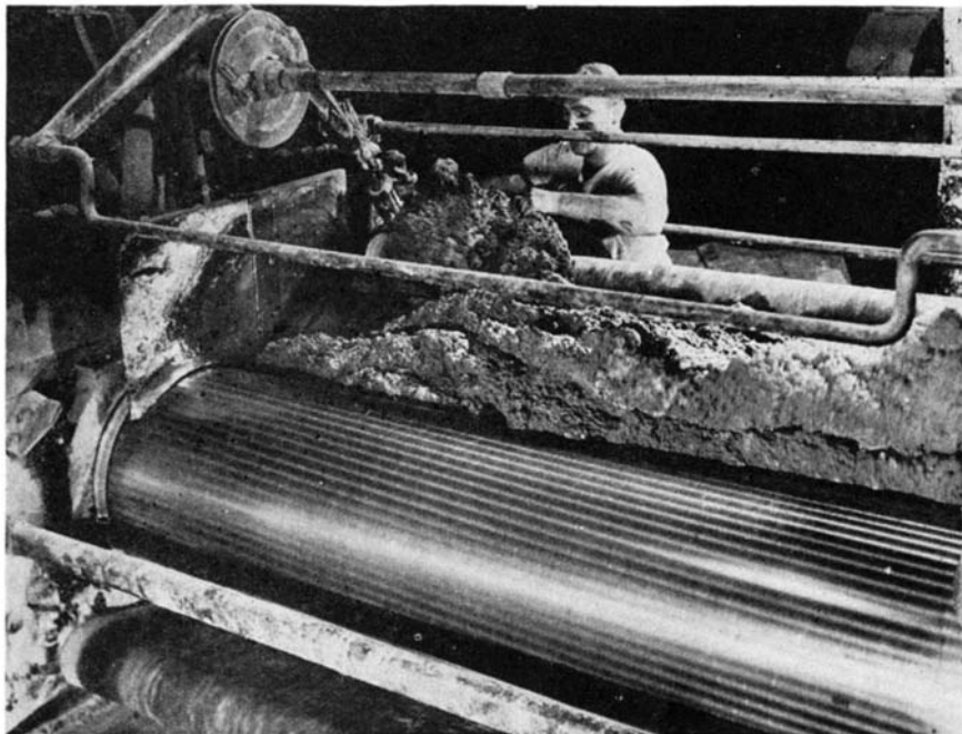
The mixing mill. Steam-heated rolls knead and mix scrap being processed
