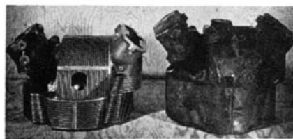
Forged cylinder head; rough stock
