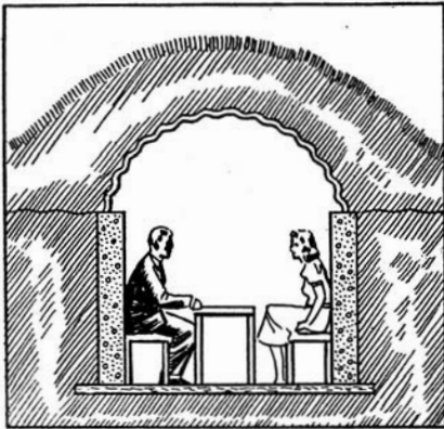
Above: Anderson type of domestic shelter. Inexpensive and effective against blast and splinters. Poor on heat, sanitation. Reproduced by permission from "What the Citizen Should Know About Civilian Defense," by Messrs. Binger and Railey, published by W. W. Norton & Co.
