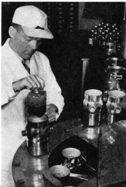
Removing bottles from centrifuge which whirled them at 2500 rpm
