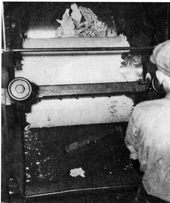
Preparing a soybean plastic molding compound
