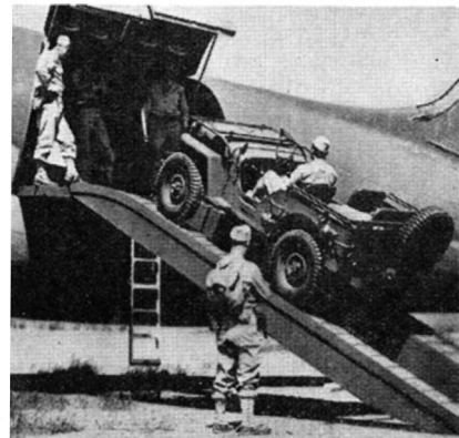
Special ramp permits rapid entry and exit of soldiers and vehicles
