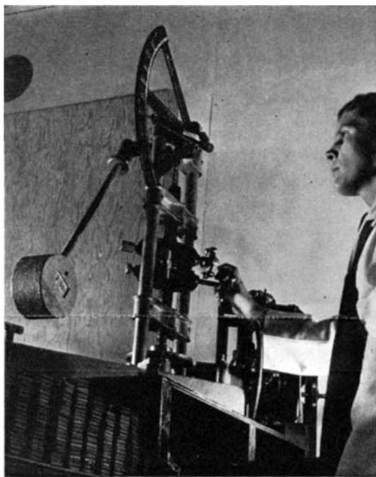
In this plywood testing machine, specimens are pulled apart to show relative strengths of the wood and glue. The wood must rupture before the glue
