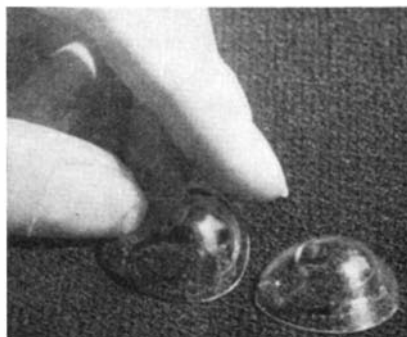
From the molds just made, the final contact lenses are cast in plastic and finished, each as individual as a fingerprint, are each a precise fit
