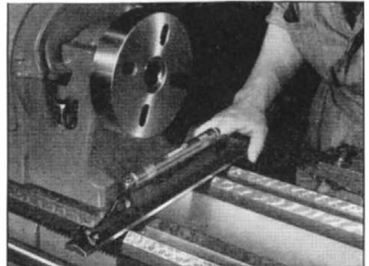
Check every lathe periodically to see that it is level
