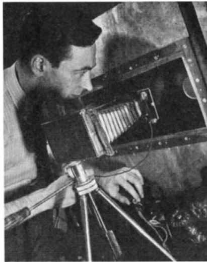
Right: Camera set-up for analyzing liquid sprays. Above: "Portraits" of flying water droplets, "stopped" by a ten millionths of a second spark flash
