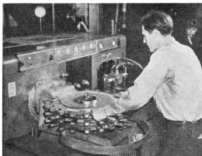
Quenching the induction-heated teeth on three high-speed tractor sprockets
