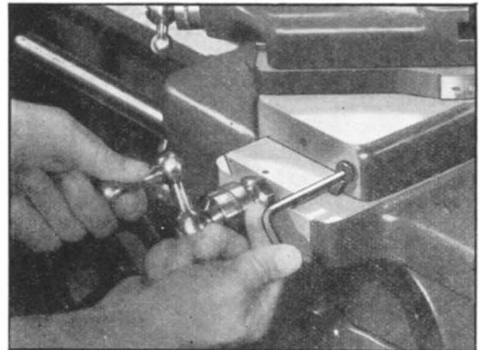
Adjust the dovetail gibs to insure accurate work
